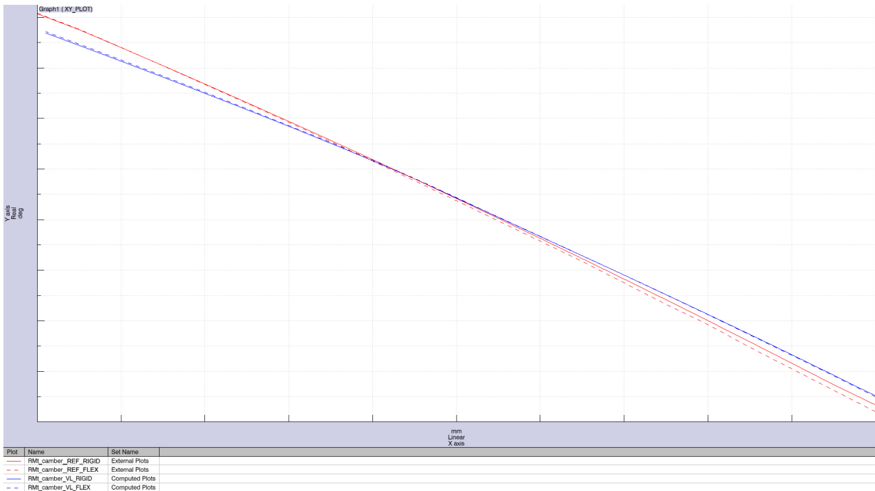
Figure 4.3.3: Camber angle over opposite vertical wheel displacement
