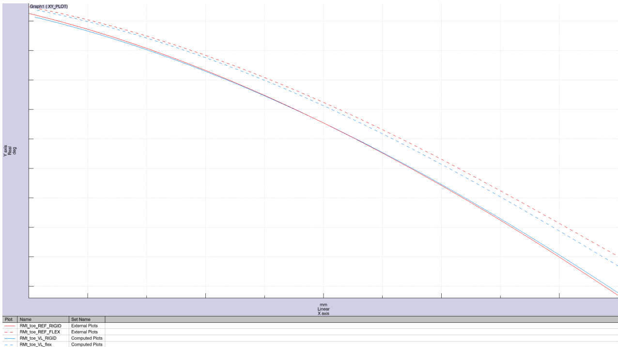
Figure 4.2.3: Toe angle over opposite vertical wheel displacement
