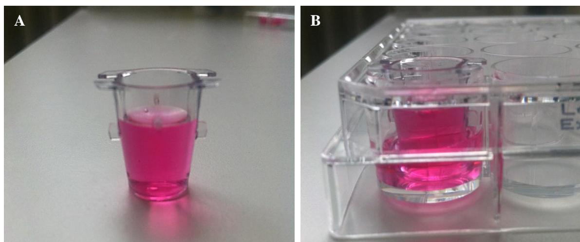
**Figure 4.** Images of the cell culture insert and 24-well plate. **A)** Image of a cell culture insert with growth medium. **B)** Image of a cell culture insert inside a well in a 24-well plate. Growth medium is placed in both the insert and the well so that cells cultured inside the insert are surrounded by growth medium.
