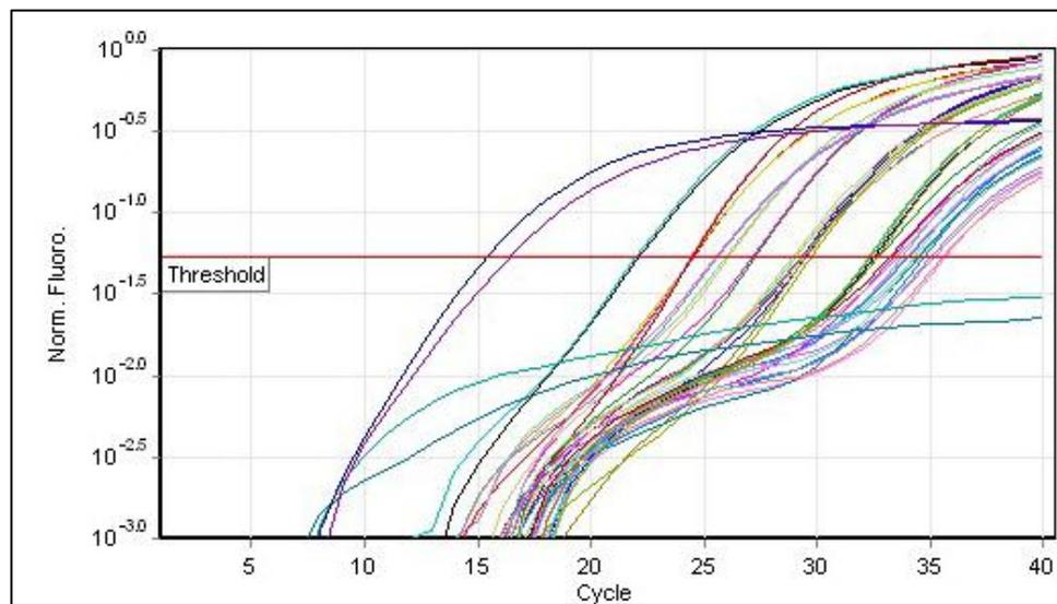
**Figure 3.** Example graph obtained from a RT-PCR run in which a threshold line is set. Normalized fluorescence is plotted against the number of cycles. Duplicates of each sample were run and the fluorescence threshold value is set to cross the sample lines in the linear phase. The  $C_T$  values are read on the x-axis specifically where each sample line crosses the threshold line.
