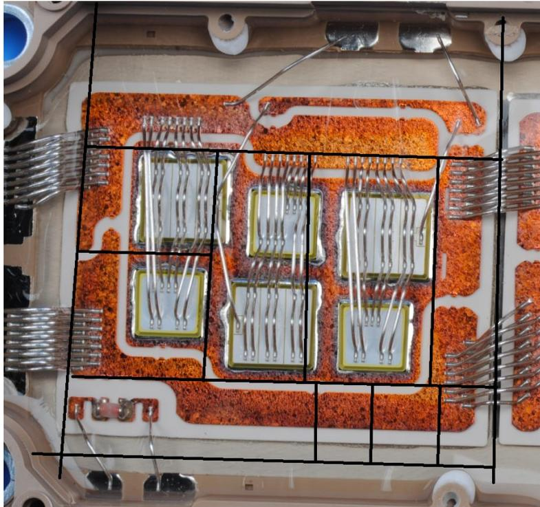
Figure 18: The cutting of the modules that are inspected in epoxy samples.
