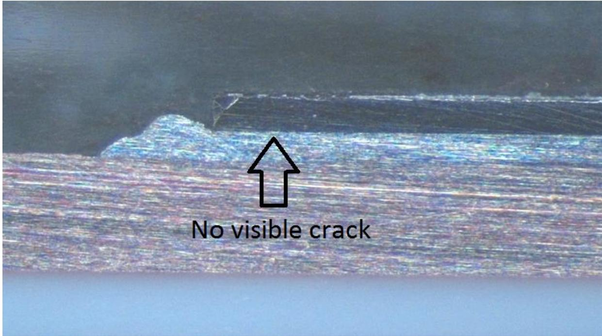
**Figure 21: Same chip as in Figure 20 but after polishing.**
