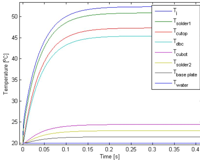
**Figure 12: The temperature increase calculations for each layer when heating up.**
