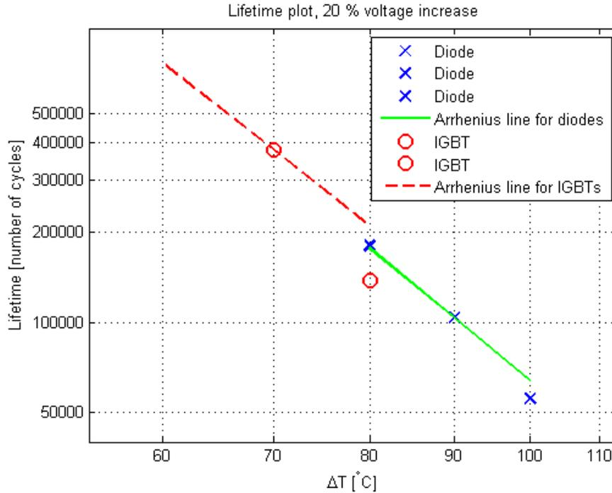
Figure 29: Lifetime of the diodes and the IGBTs together with the lifetime curve from ( 2 ).
