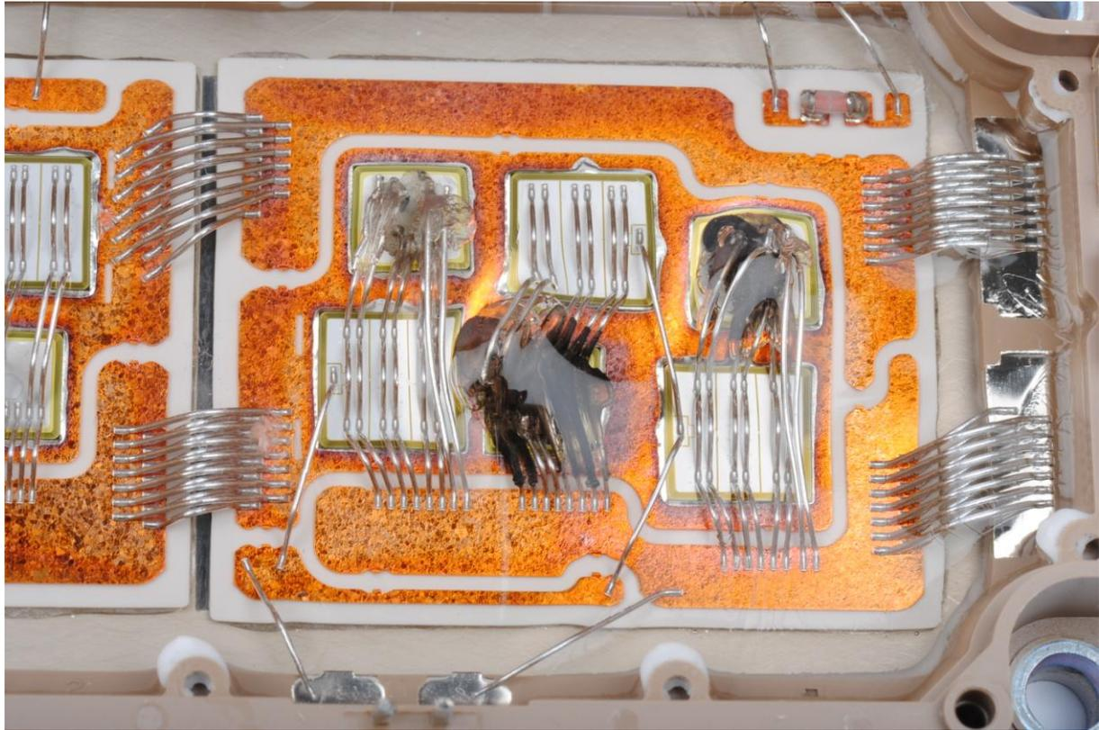
**Figure 17: Fuji module sample number 7, this is the first diode to break at 300A.**
