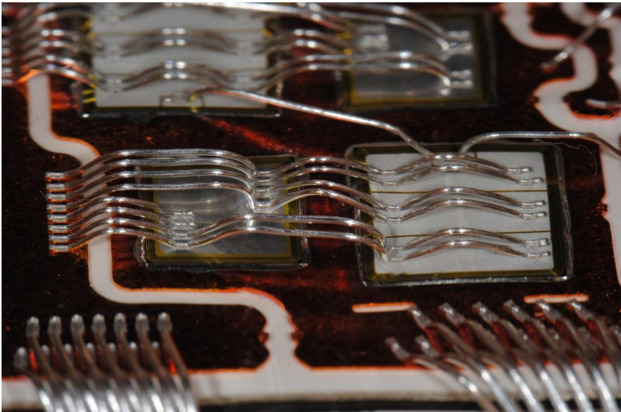
Figure 6: The bond wires to the diode and IGBT of Fuji 2MBI300VN-120-50.
