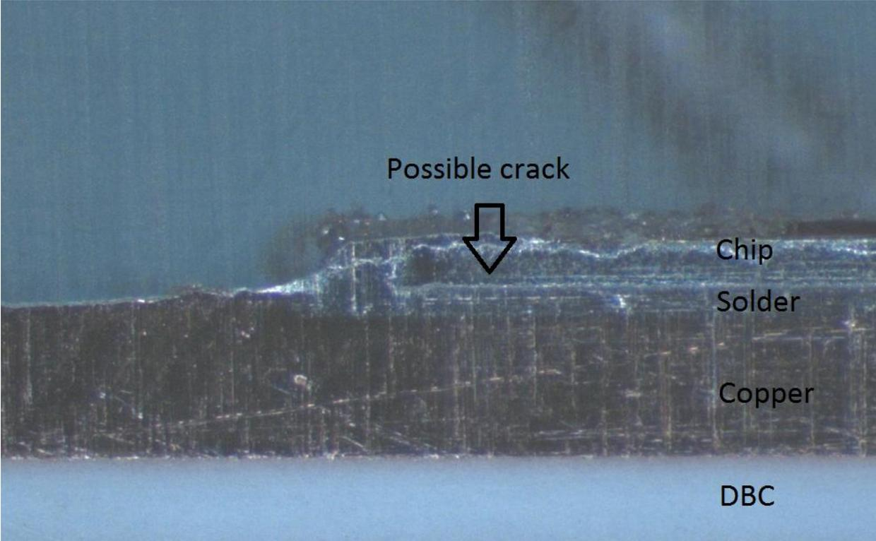
Figure 20: A potential crack between the chip and the solder layer, the sample is only grinded roughly.
