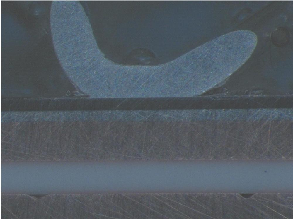
Figure 22: Bond wire to a diode in module number 6.
