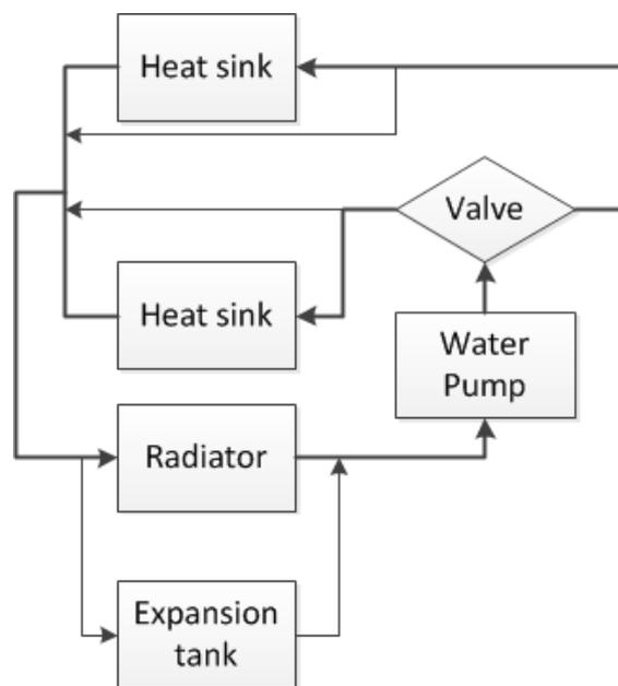
Figure 15: Block diagram of the cooling water system.
