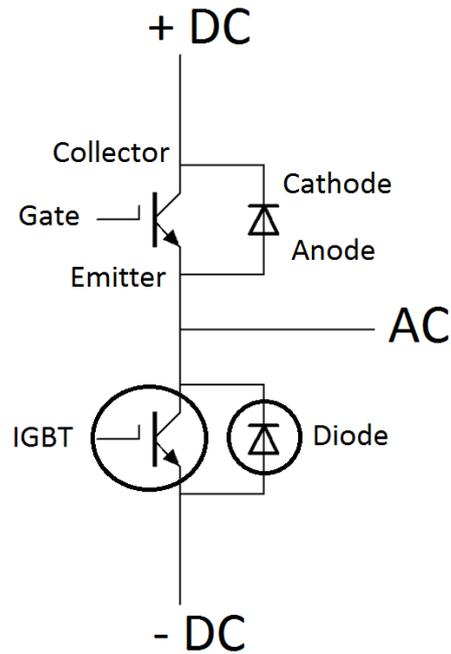
Figure 3: One phase leg of an IGBT.
