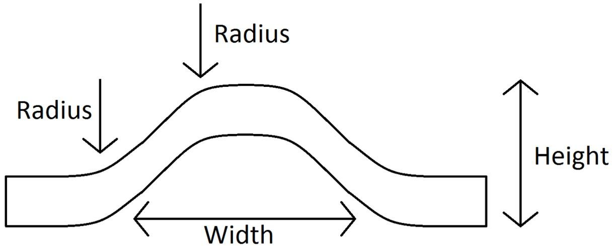
Figure 7: Schematic view of a bond wire.
