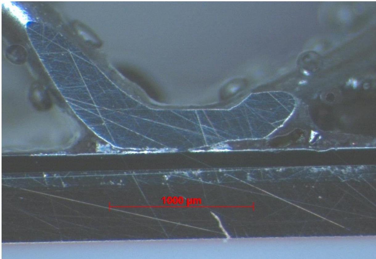
Figure 23: Bond wire to an IGBT in module number 6, cracks can be seen between the bond wire and the chip.
