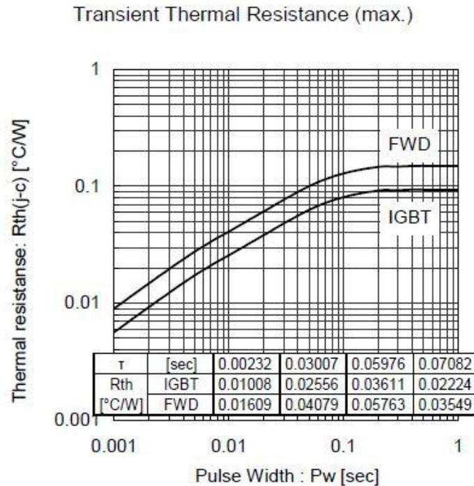
Figure 10: Transient thermal resistance for Fuji 2MBI300VN-120-50 [21].
