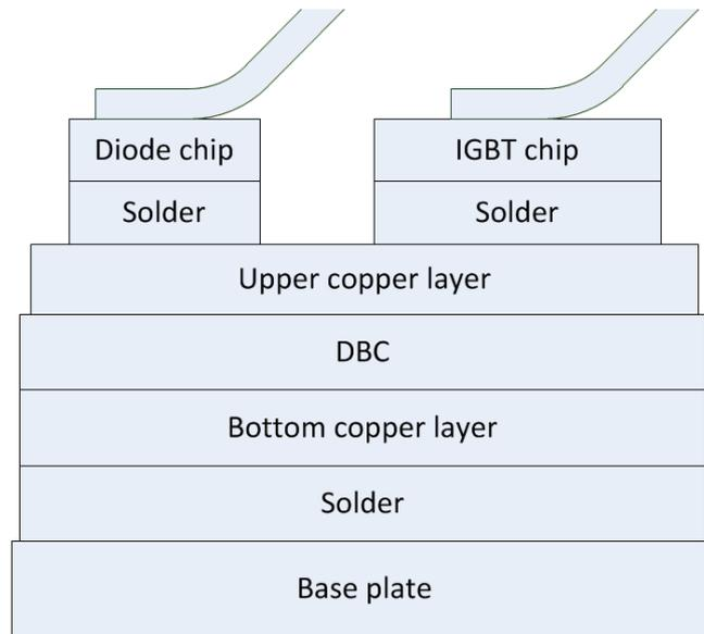
Figure 5: A sectional image of a PE module.
