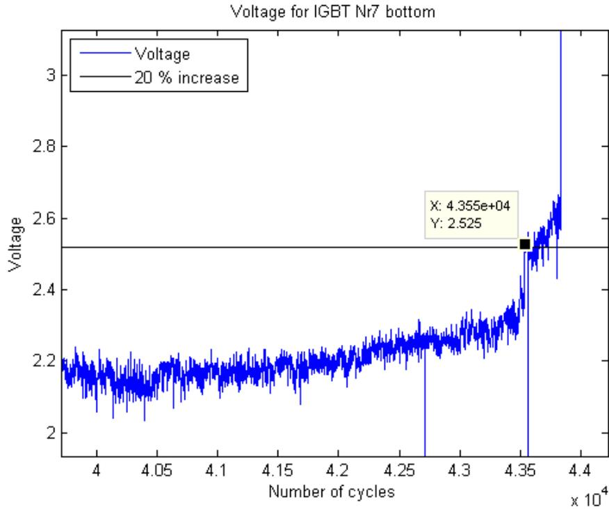
Figure 26: Voltage for the bottom diode in module number 7.
