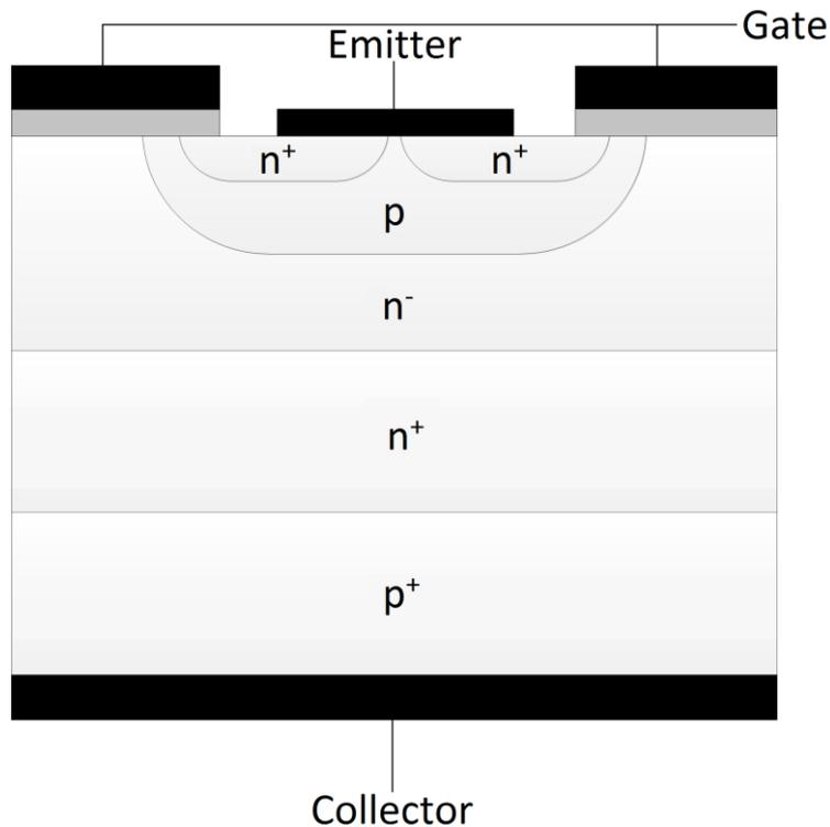
Figure 1: The semiconductor layers in an IGBT chip [3].
