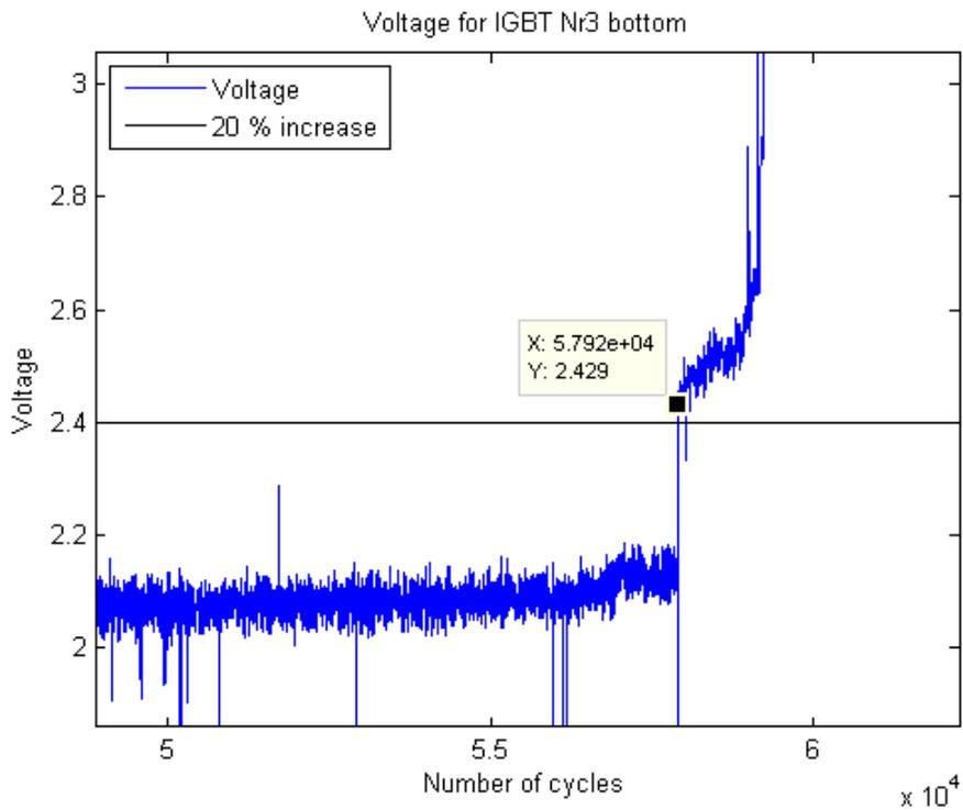
Figure 27: Voltage for the bottom diode in module number 3.
