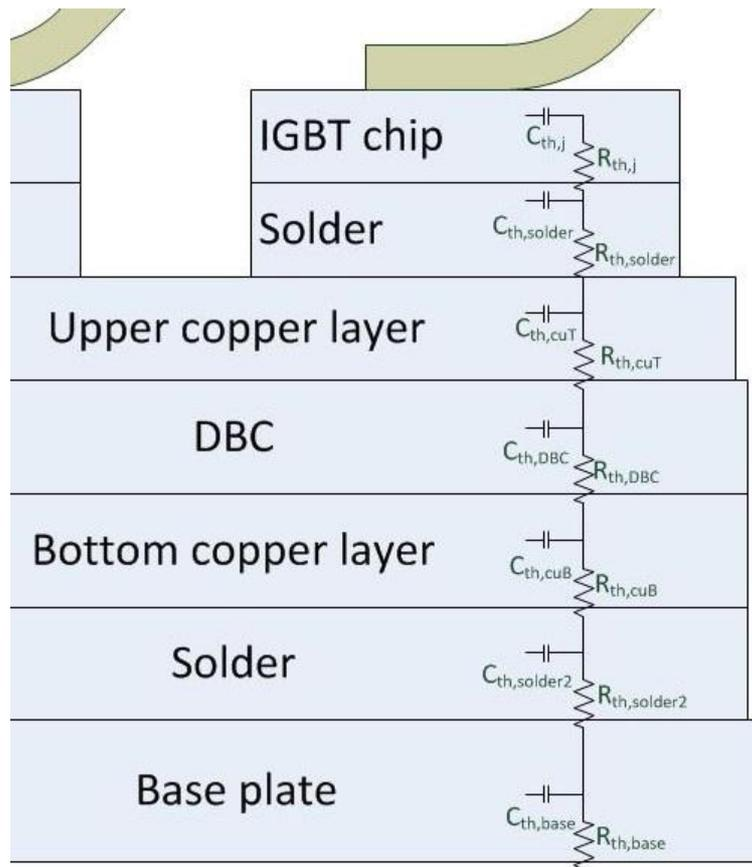
**Figure 9: The thermal capacitances and resistances in the system.**
