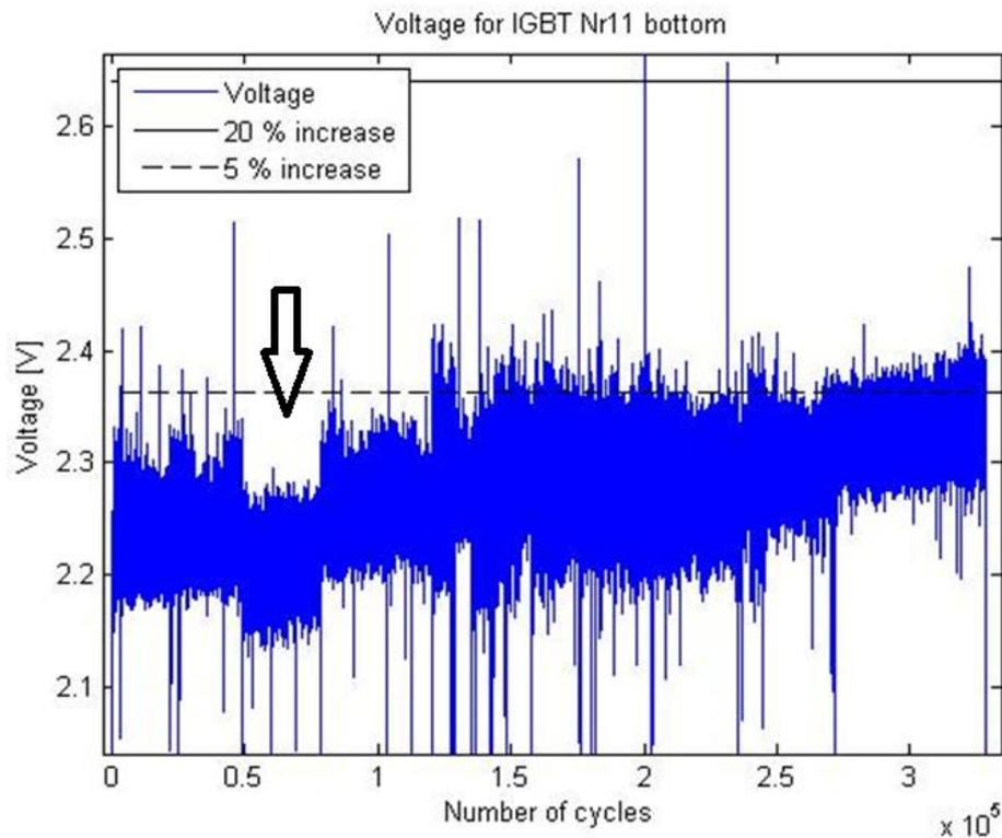
Figure 28: Voltage increase during the whole lifetime for the bottom IGBT in module number 11.
