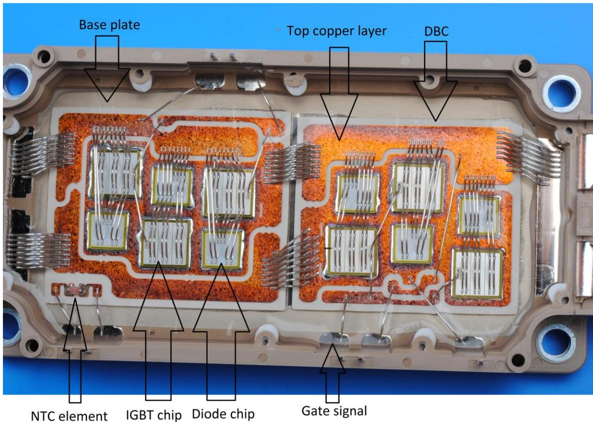
**Figure 4: A PE module with three chips for each diode and IGBT.**
