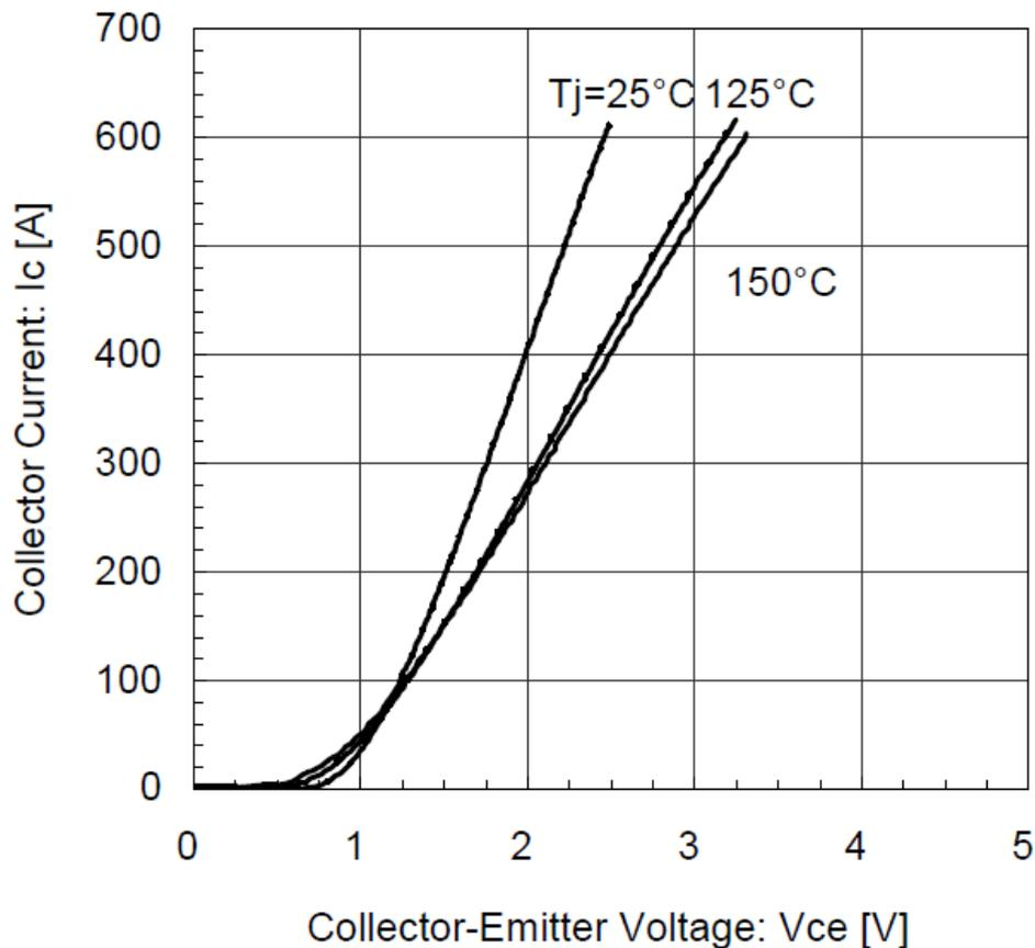
Figure 11: The collector-emitter voltage dependency of the current [21].
