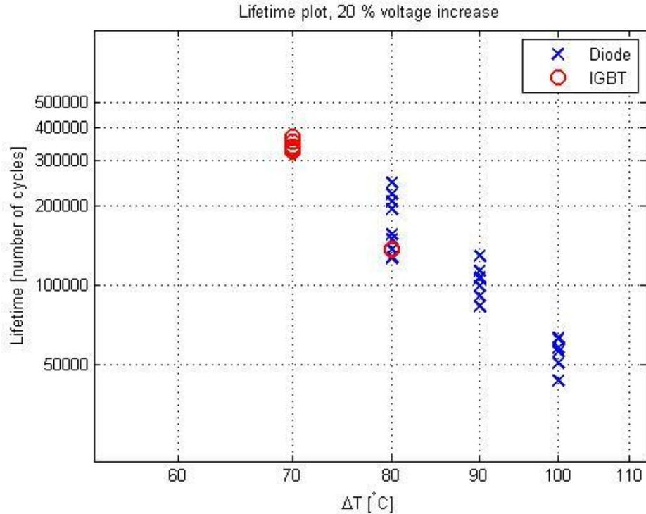
Figure 30: All failures of Diodes and IGBTs.
