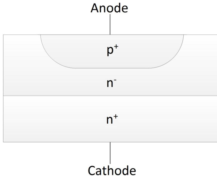
Figure 2: The semiconductor layers in a power diode chip.
