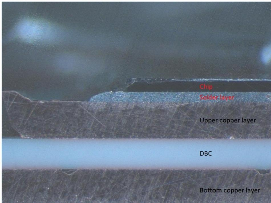
Figure 19: Diode chip for sample number 3, no solder delamination can be seen.
