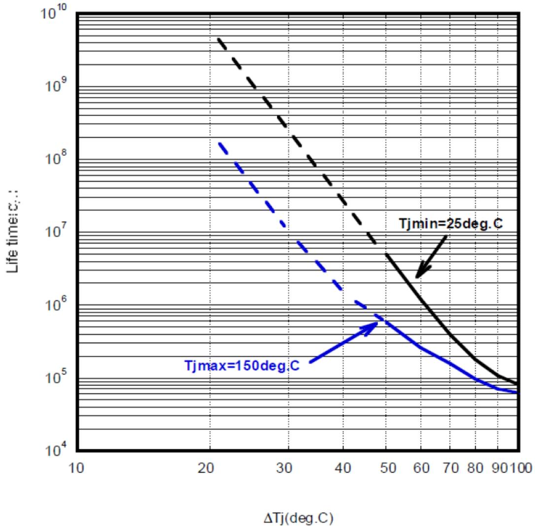
Figure 8: The lifetime for different  $\Delta T_j$  from datasheet to Fuji 2MBI300VN-120-50 [17].
