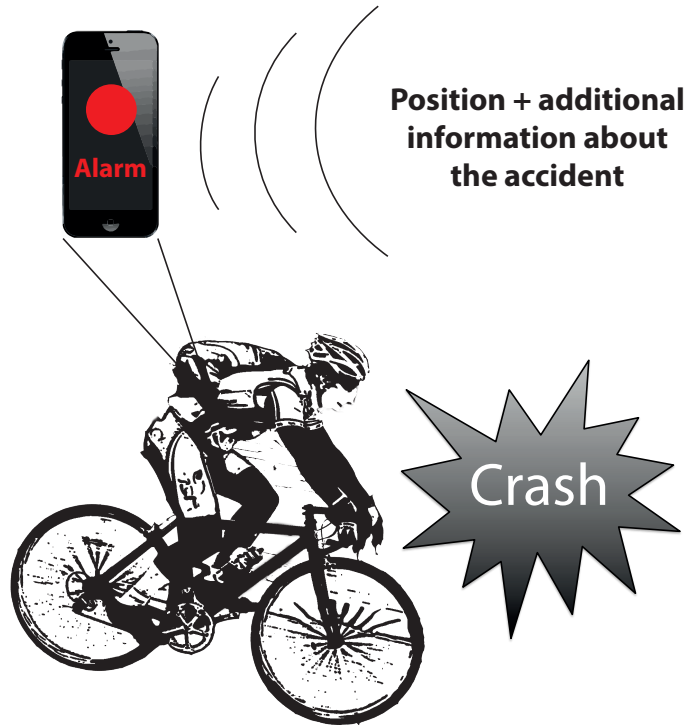
Figure 1. The principle of eCall functionality for cyclists implemented on a smartphone.
