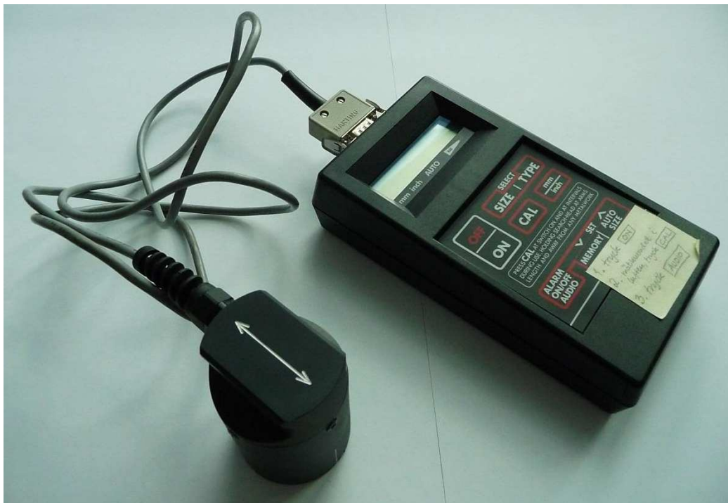
Figure 4.2 Micro Covermeter, used to measure the cover thickness
