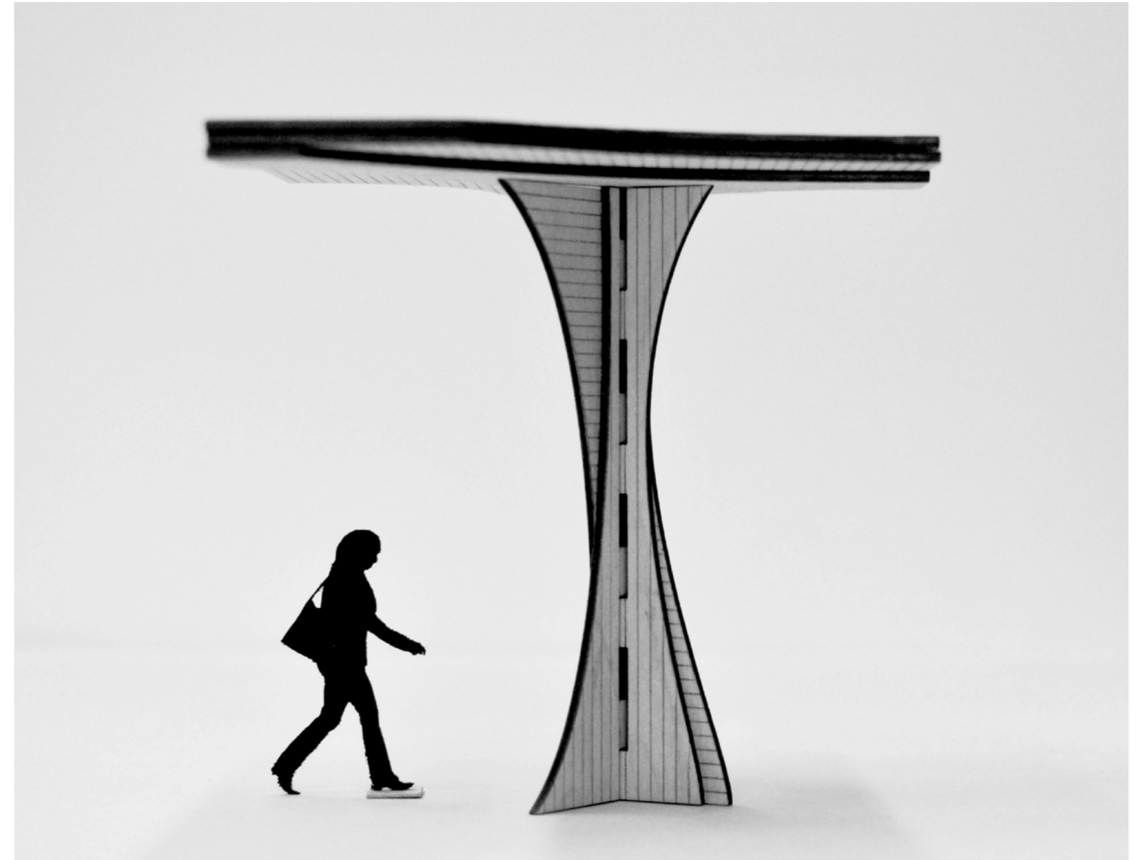
PROTOTYPING - Layering of the CLT roof -
