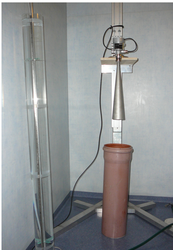
Fig. 7 The plastic tube with the bubble chamber lowered into the water (to the left) and the radar sensor (to the right) being tested in one of the showers at the observatory.
