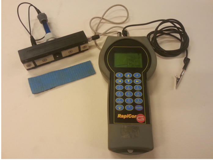
Figure 4.21: RapiCor handheld device
