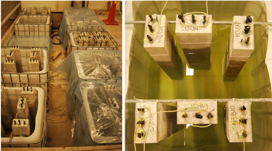
Figure 4.16: Beams subjected to partial immersion in 10 % chloride solution
