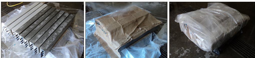
Figure 4.13: Storage process of the beam specimens for curing
