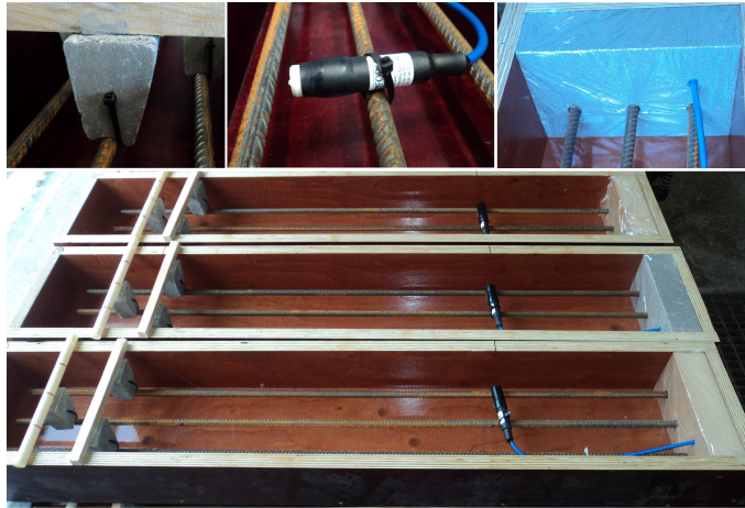
Figure 4.12: A detail of a fibre-reinforced concrete spacer (top-left); an embeddable reference electrode ERE20 (top-centre); insulation of reinforcing bars with hard-foam (top-right); and a general view of the formworks (bottom)
