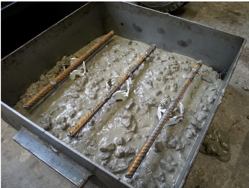
Figure 6.4: Production process of specimens for the galvanic corrosion experiments
