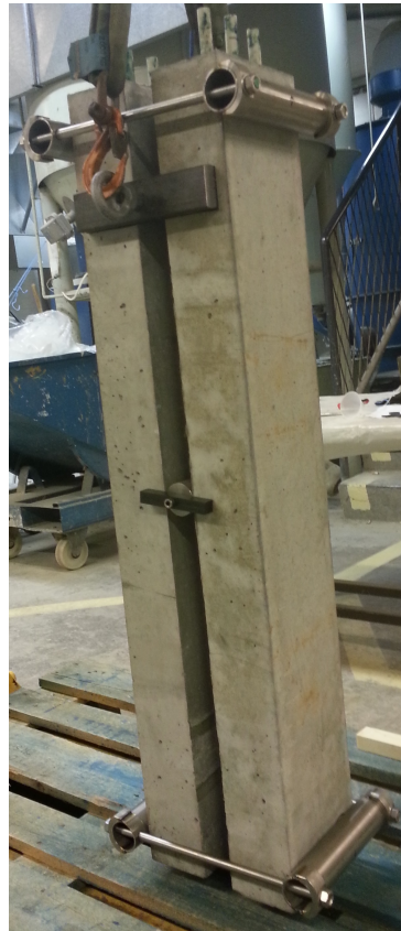
Figure 4.15: Setup for sustained loading, measurements in mm
