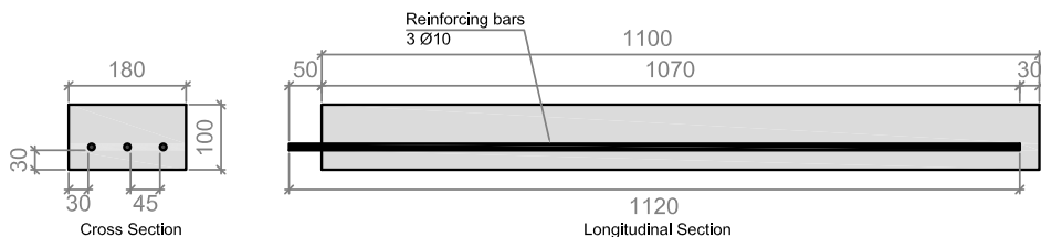
Figure 4.11: Specimen geometry, measurements in mm
