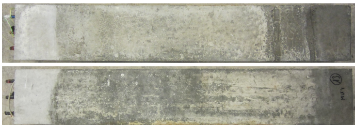
Figure 7.12: State of the beam surfaces for the different series after a year of cyclic exposure to chloride solution.
