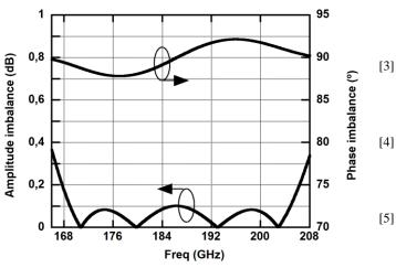
Fig. 5. Simulated through and coupled performance of the modified periodical waveguide hybrid [5].
