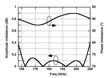
Fig. 6. Measured through and coupled performance of the modified periodical waveguide hybrid [5].
