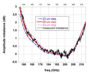
Fig. 4. Simulated performance for different step length lengths.
