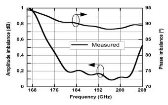
Fig. 3. Measured amplitude and phase imbalance of the synchronous hybrid shown in Fig.2.
