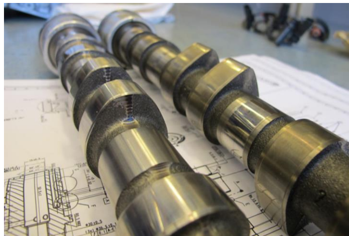
Figure 15 – LIVC & original intake camshaft
