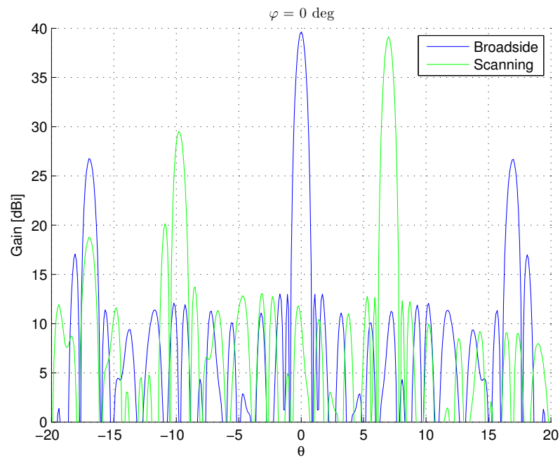
Figure 4.25: Scanning is shown for the \varphi = 0^\circ plane, using the large pyramidal horn for the small spot size.
