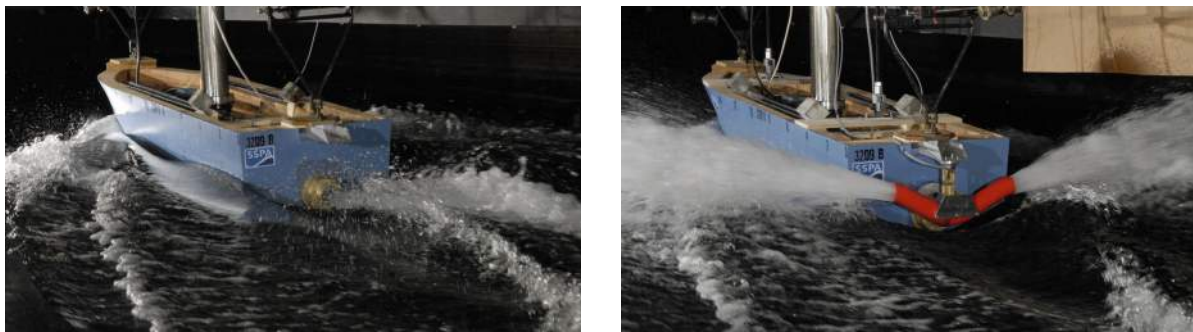
Figure 8.8 self-propulsion test at SSPA at Fn = 0.8 (left: without the T-junction, right: with the T-junction)
