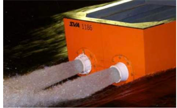
Figure 4.7 Model scale ATHENA with working waterjets (ITTC 2008)
