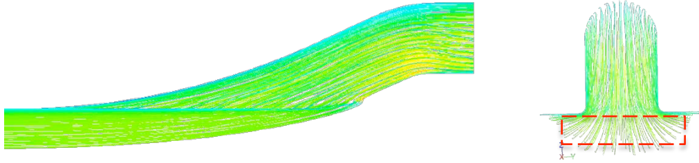
Figure 3.5 Backward tracing of the streamlines for obtaining the capture area; left: side view and right: stern view. The dashed line shows the rectangular capture area.
