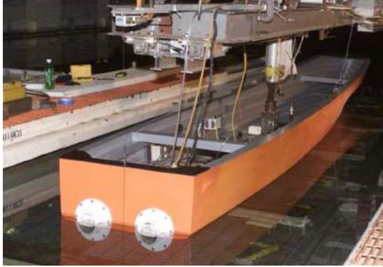
Figure 4.6 Model scale self-propulsion test setup (ITTC 2005c)
