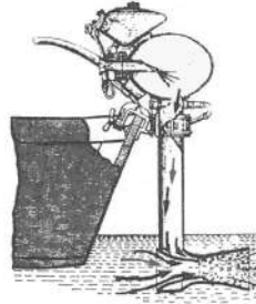
Figure 1.6 Sketch by Schult of H. J. MacCollum's (1946) Pulse Jet Outboard (Schult 1974)
