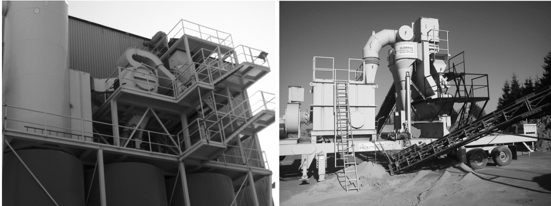
Figure 32. Investigated air classifiers, to the left two-stage air classifier and to the right mobile air classifier.
