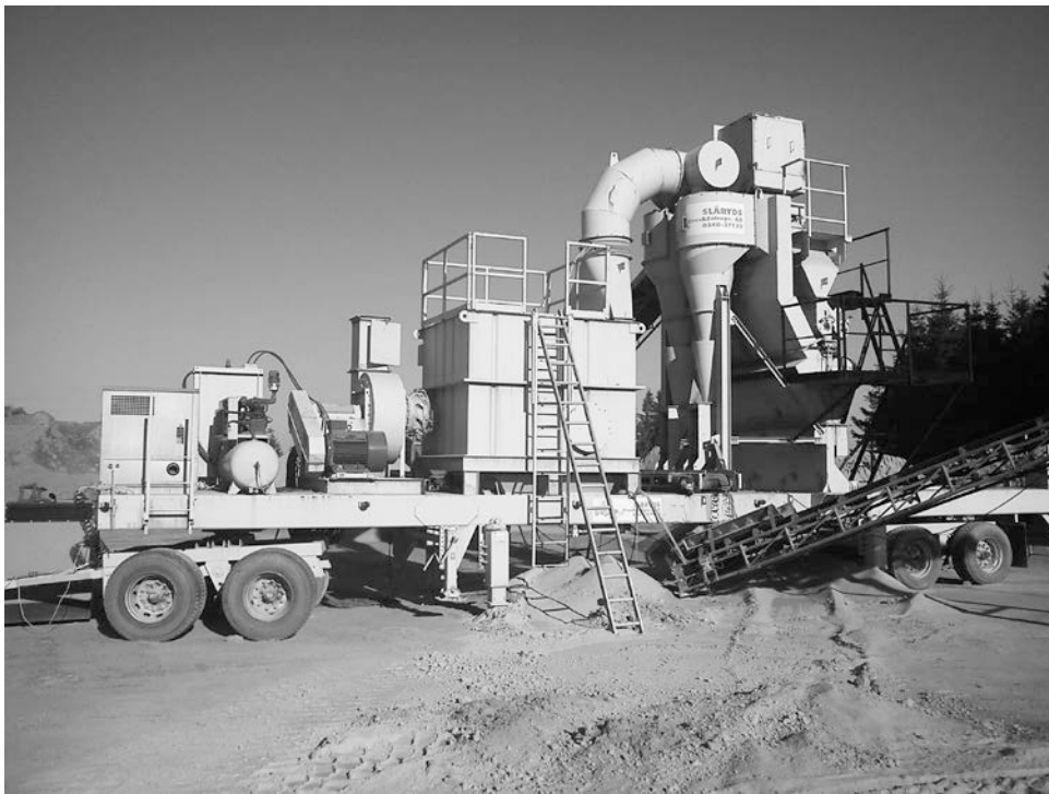
Figure 64. Mobile air classifier with air filter.
