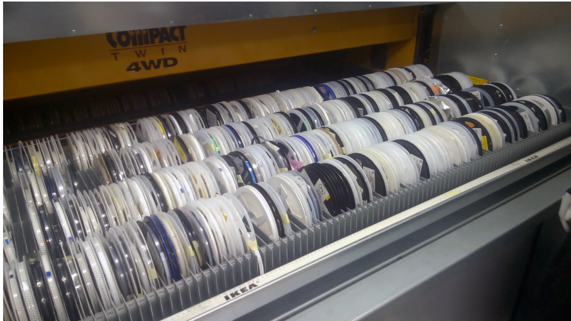
Figure 4.2: A shelf from the storage elevator with roll components
