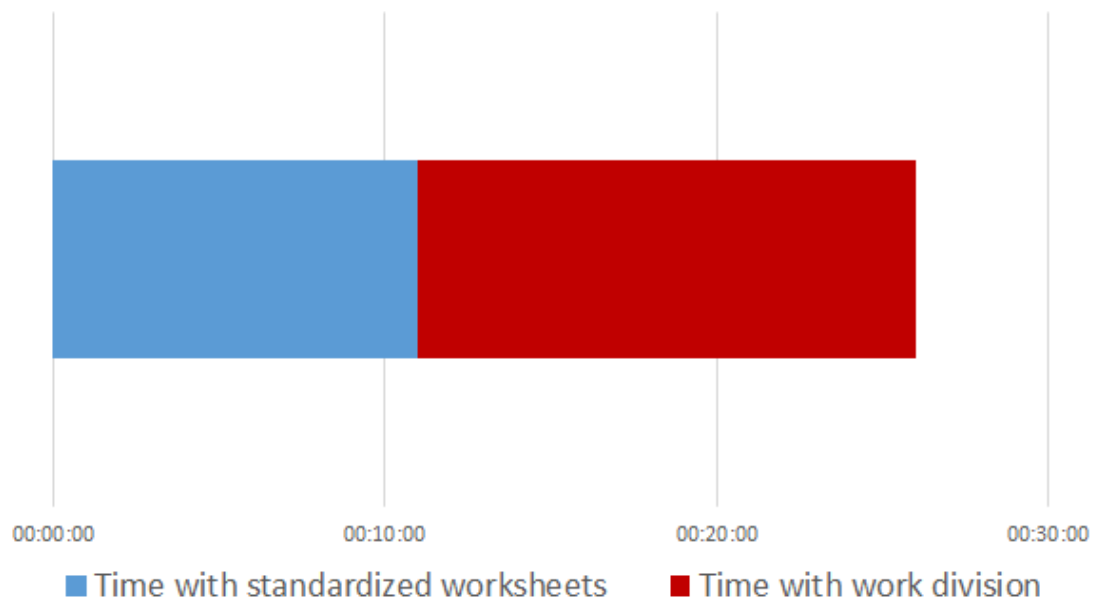
Figure 6.2: The reduction of changeover time, using the standardized worksheets
