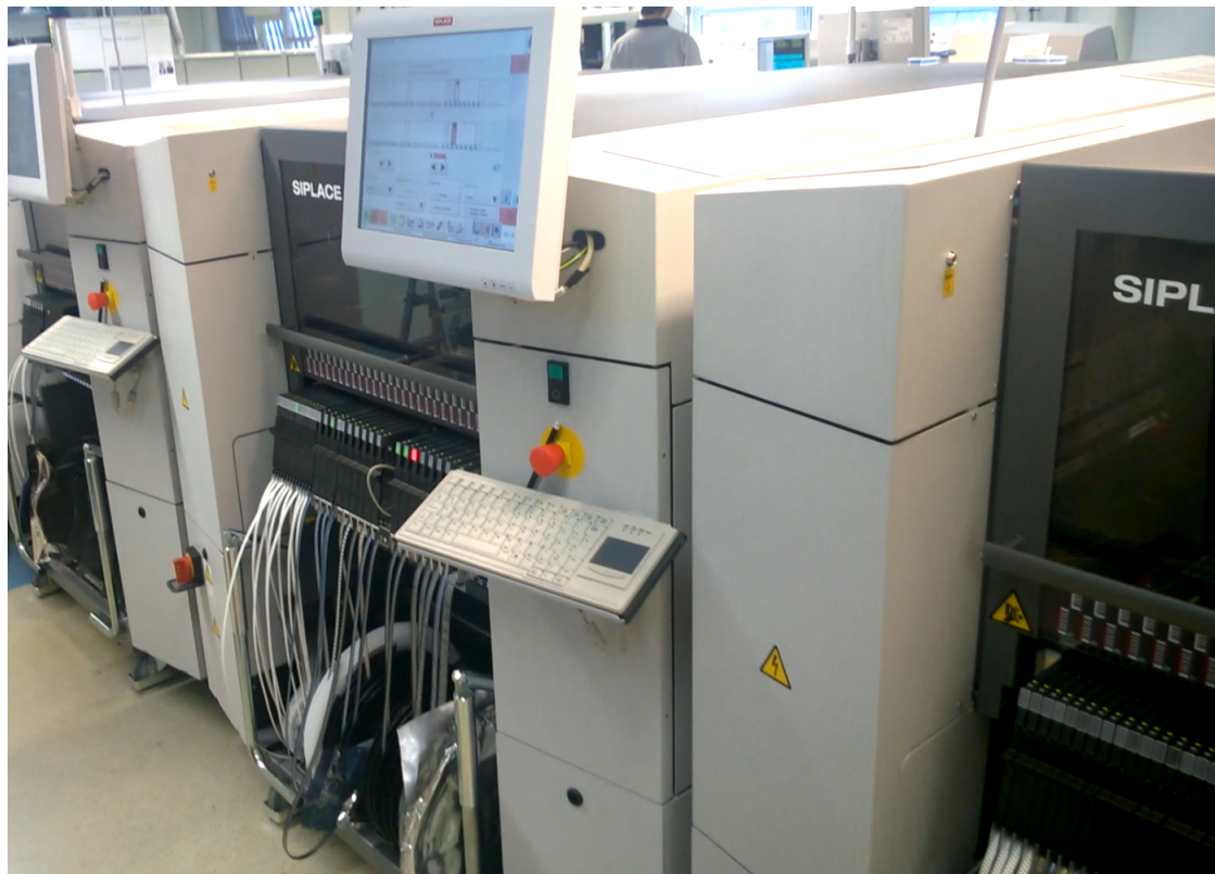
Figure 1.4: One ASM machine with mounted roll components
