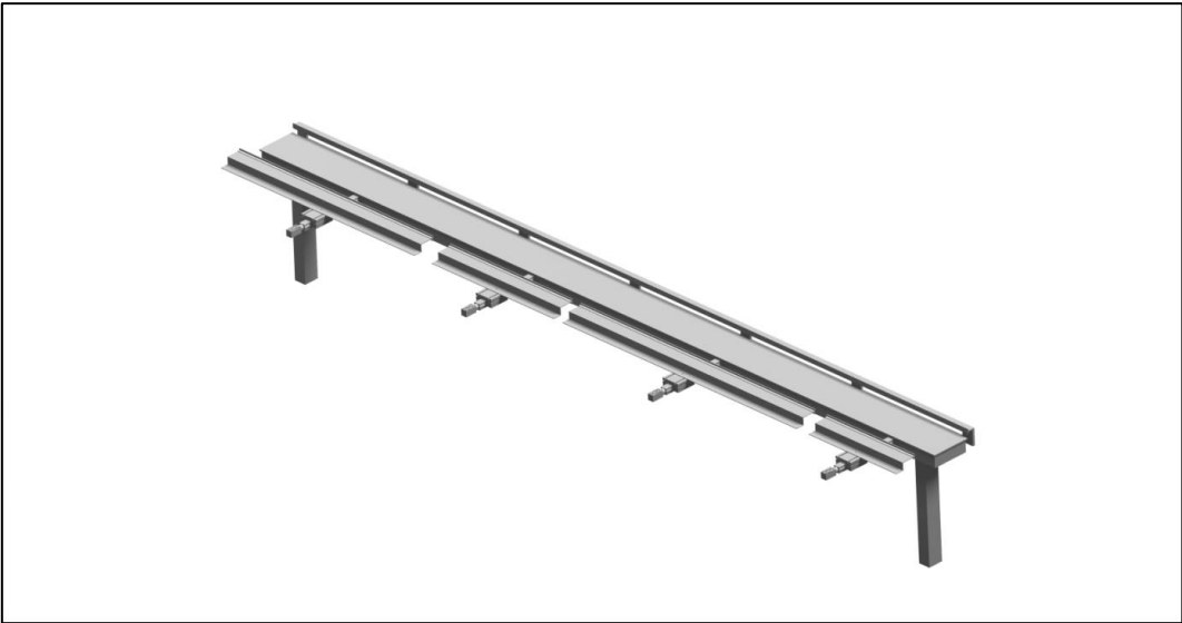
Figure 24: A picture of guide rail 1-4 with motors.
