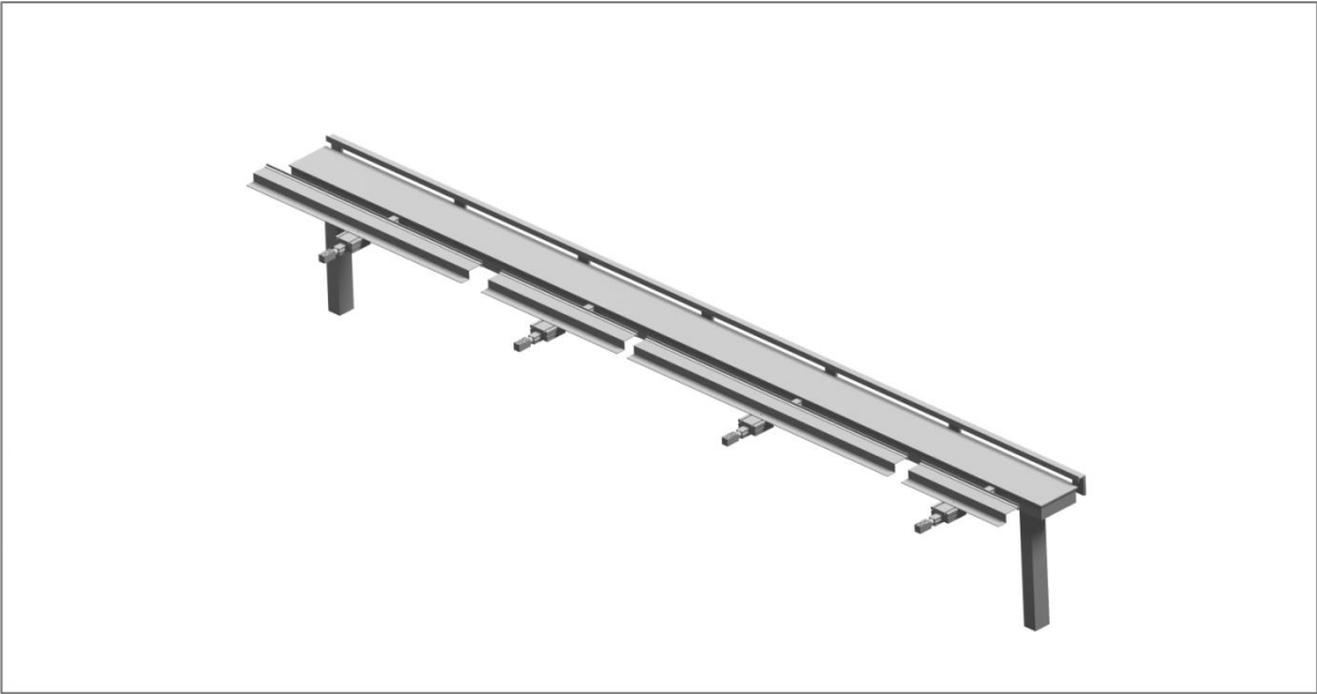
Figure 17: Illustration of guide rail 1-4 with linear actuators and motors.
