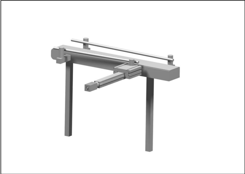
Figure 29: A picture of guide rail 6 with motor.
