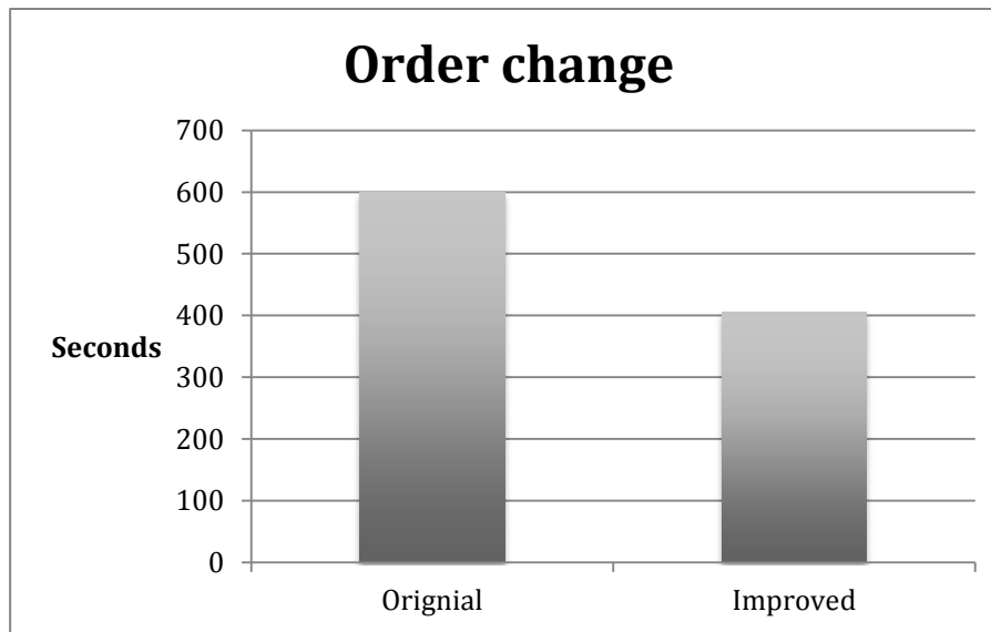
Figure 29: Comparison of order change time between original and improvement
