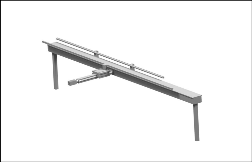
Figure 32: A picture of guide rail 7 with motor.
