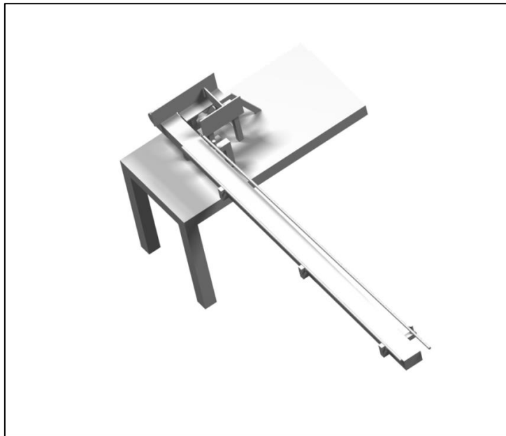
Figure 40: A picture of guide rail in the warehouse with hand wheel.
