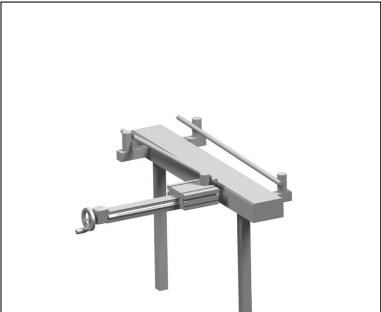
Figure 30: A picture of guide rail 6 with hand wheel.
