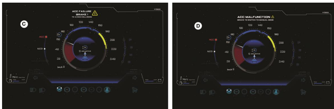
Fig 45: C- ACC failure mode when in critical situation. D- ACC failure mode when in non-critical situation.
