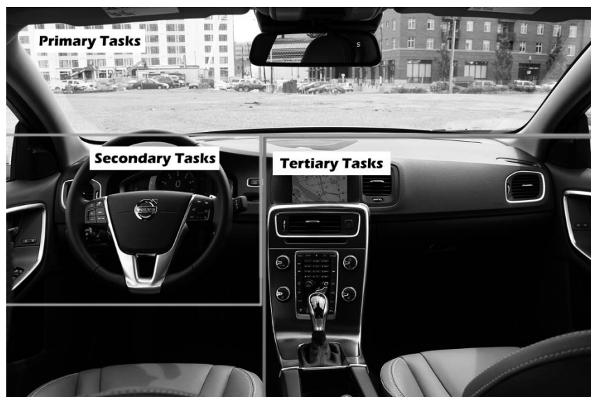
Figure 9: Distribution of primary, secondary and tertiary tasks in a driver cockpit. Adapted from ‘A Survey of Challenges Related to the Design of 3D User Interfaces for Car Drivers’ (Tönnis et al. 2006). Background image from Braun (2014).
