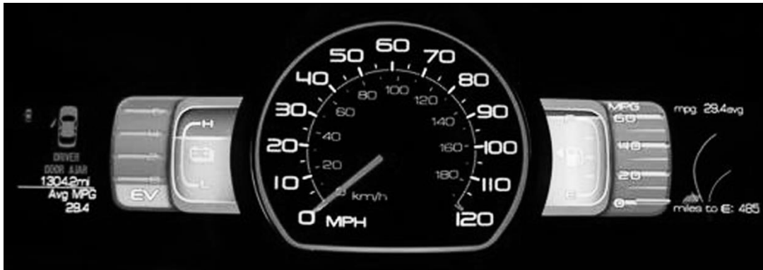
Figure 11: Ford Fusion Hybrid instrument cluster. Adapted from Huffman (2010) Ford fusion hybrid instrument cluster .
