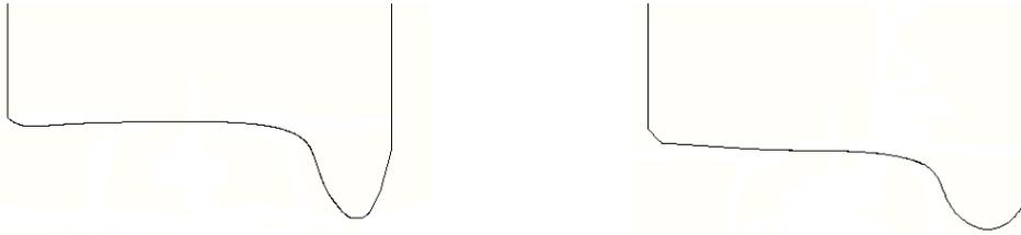
Figure 15 Wheel profiles, to the left a hollow worn and to the right a new conical shaped wheel, S1002. As seen in the pictures the flange is thinner and the flange angle is larger for the hollow worn profile compared to the new S1002 profile.
