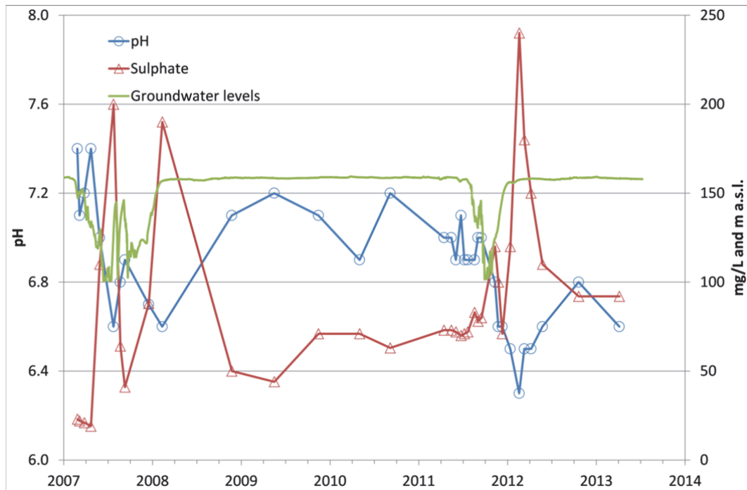
Figure 9.4. Concentrations of SO_4^{2-} , pH and groundwater levels in BP08. There was an increase in SO_4^{2-} concentrations and subsequent decrease in pH during time periods with groundwater recovery, such as after the construction of the eastern (2007/2008) and western (2011/2012) tunnel tubes through the study area.
