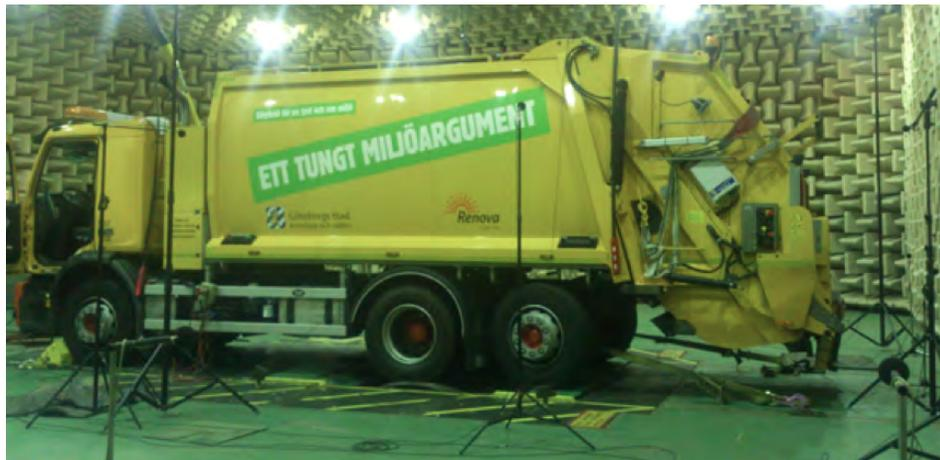
Figure 3.2.: An overview of the recording setup for the Volvo FE Hybrid truck in a semi-anechoic laboratory [3].
