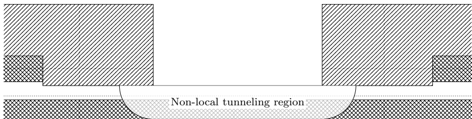
Figure 3.13: Extent of the non-local tunneling region in which the energy band structure is computed and used to compute the probability of tunneling.
