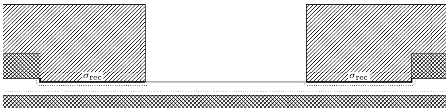
Figure 3.7: Illustration of the placement of surface traps at the \text{Si}_3\text{N}_4/\text{InAlAs} interface.
