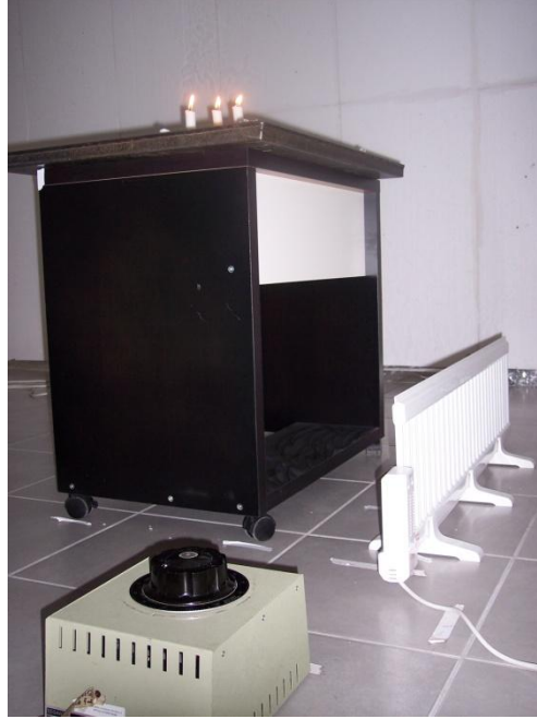
Figure 22. Disturbance sources during experimental studies. Additionally, a temporary wall of Styrofoam can be seen in the background.
