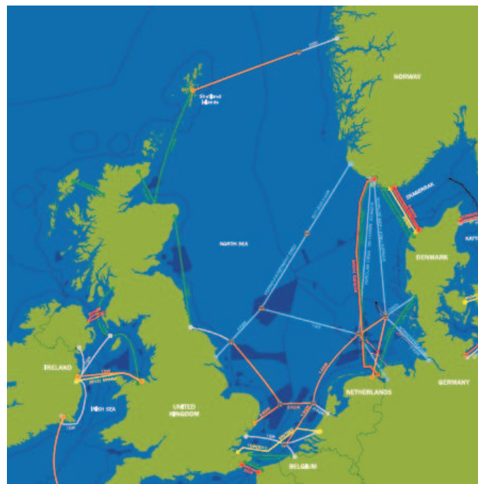
Figure 2.8: Vision of HVDC grid in the North Sea area proposed by EWEA. Existing HVDC links in the area are also indicated in red in the figure [42].
