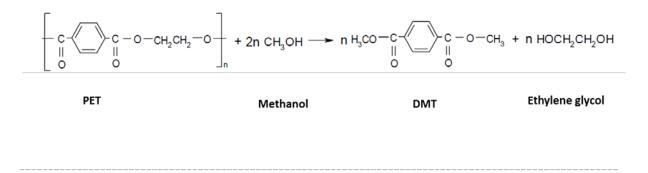
Figure 4 : Chemical equation of methanolysis of PET
