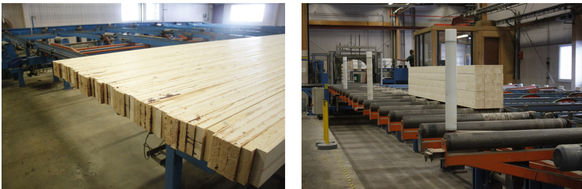
Fig 2.15 New glulam and japanese wood products in the production line at Martinsons factory in Bygdsiljum [Orstadius and Nordström 2013].
