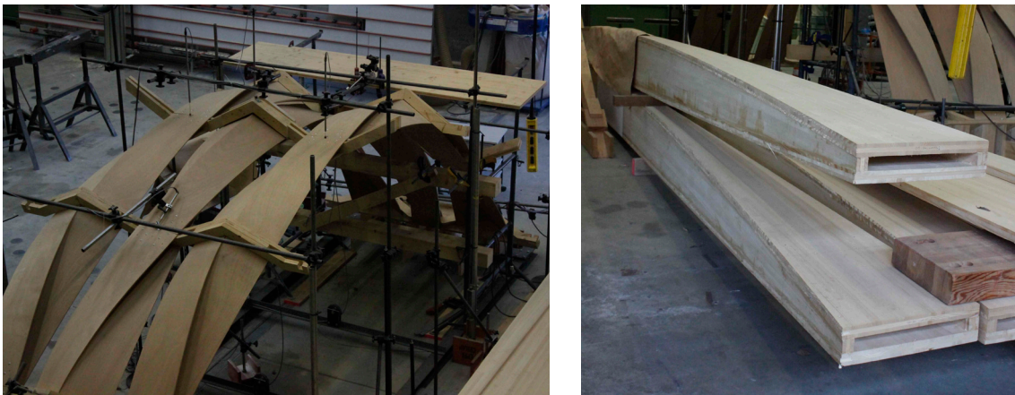
Fig 2.14 Images from study visit in Weinand's studio at IBOIS. Timber is used to create innovative structural forms and large scale physical testing is conducted to verify digitally modelled ideas. [Nordström and Orstadius, 2013]
