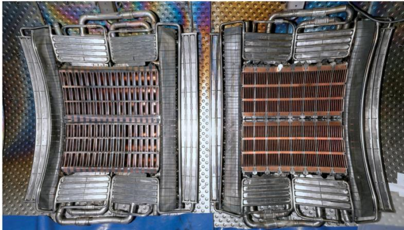
**Figure 4.3:** PAM (left) and FAM (right) launchers seen from the inside of Tore Supra.
