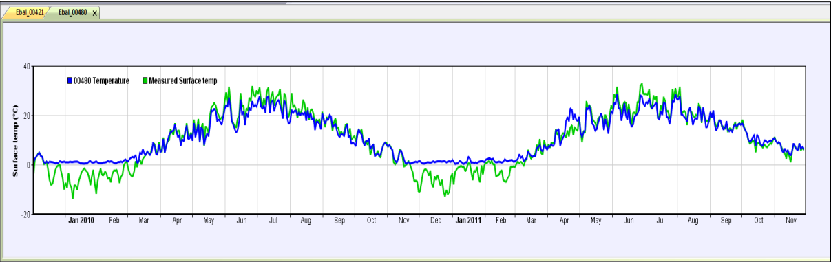
Figure 12: Static simulation with the power of 348 \text{ W/m}^2 and in the depth of 4 cm -Gothenburg
