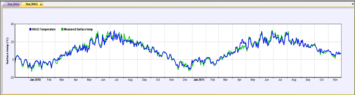
Figure 8: Measured and simulated surface temperature without using the heat source –Gothenburg
