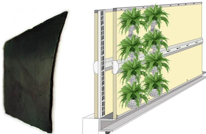
Figure 4: Vertical garden structures proposed by group C. Left to right: Image of pressed Divinycell sawdust board, vertical garden diagram.
