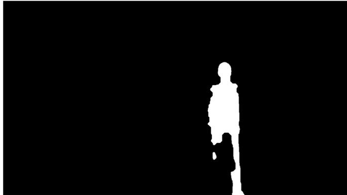
(c) Foreground pixels after noise removal with a median filter and applying opening and closing morphological operations.
