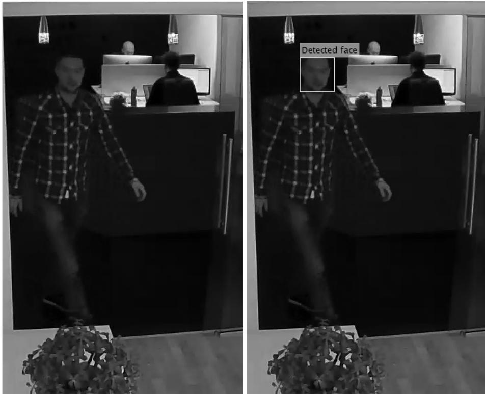
(a) Part of frame from video sequence. (b) Detected face in frame with bounding box around it.
