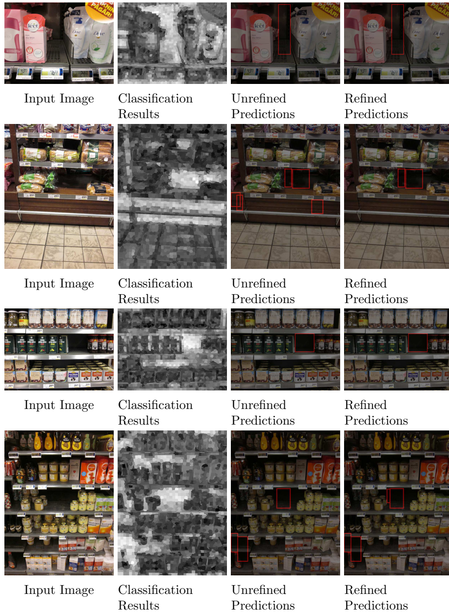
Figure A.5: Hole detection using the SVM classifier. In the second row false holes are detected beneath the shelf. Otherwise, even the unrefined predictions work quite well, due to the fact that all images contain holes.
