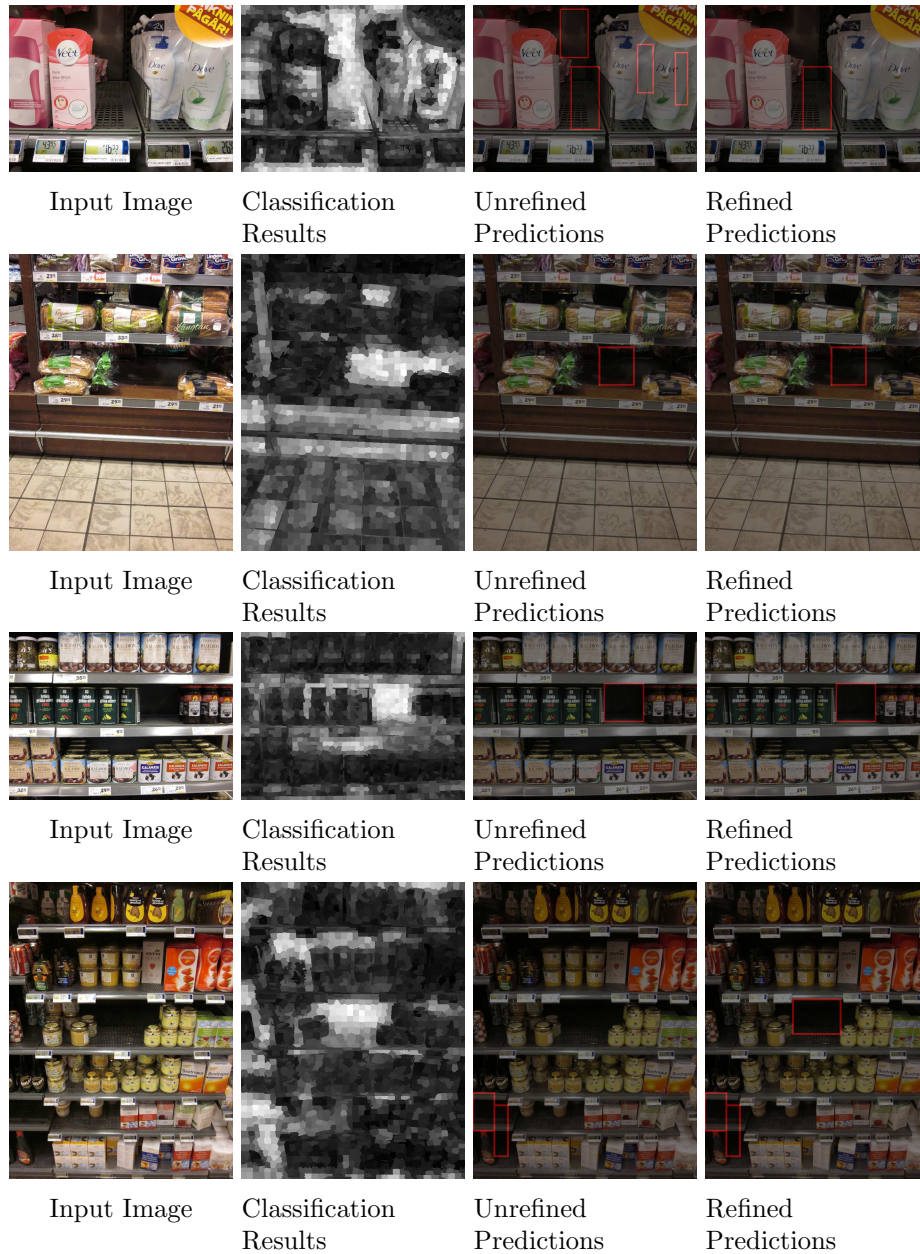
Figure A.6: Hole detection using the AdaBoost classifier. The results are quite similar to the ones obtained using the SVM classifier. Nevertheless, as can be seen in the first row, for example, the AdaBoost classifiers has more problems with false positive detections.
