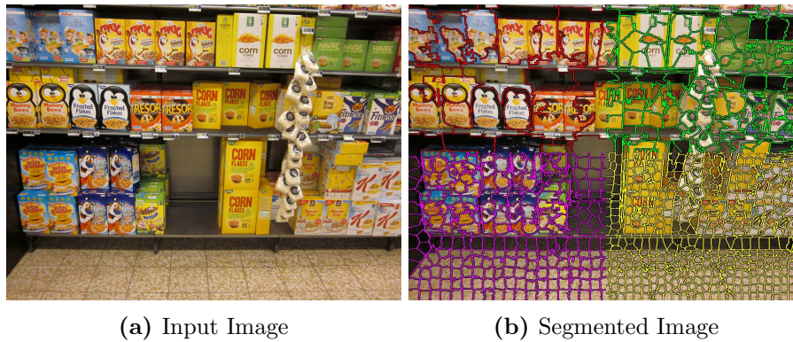
Figure 3.4: (a) Input image. An example image containing a hole and several products. (b) Superpixel segmentation of (a). Displayed are the borders of the superpixels for different numbers of superpixels in the hole image. Red corresponds to N_{sp} = 500 , green to N_{sp} = 1000 , purple to N_{sp} = 2000 and yellow to N_{sp} = 4000 .
