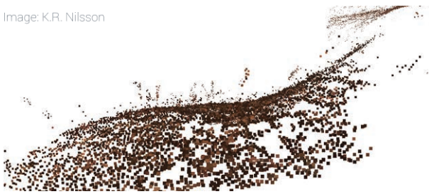
Point noise on a surface which was acquired from noisy images. To some extent noise can be reduced using Poisson Disc sampling in a software like MeshLab.
