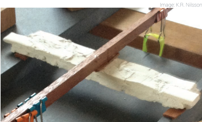
The test is performed on scale models using bricks scaled 1:10.
