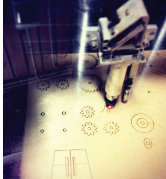
Laser cutting parts for the laser guidance machine. Plywood turned out to be a sub-optimal material for precision.
