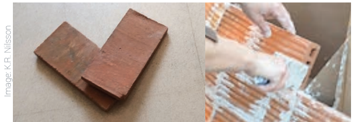
Flat tiles from Teatro la Massa and a sketch of hollow bricks with undulating sides used in a test by Block Research Group.
