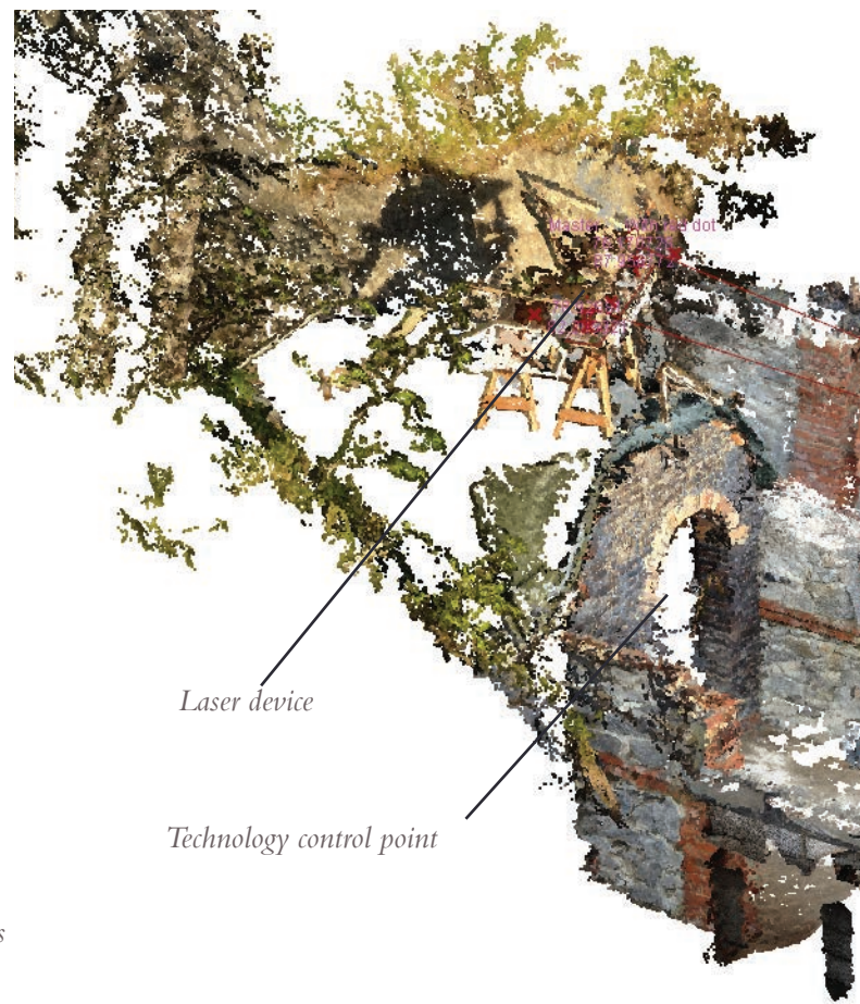
A technology control point was rigged in the room under the first vault, close enough to the laser to reach it with a USB cable.
