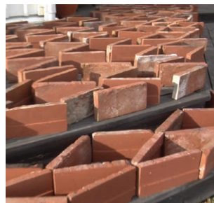
The bricks had to be cleaned to ensure a good adhesion with the mortar. Then dried for the same reason and to make them as light as possible, although only a few of them were of the light weight type made by mixing in saw dust in the clay.
