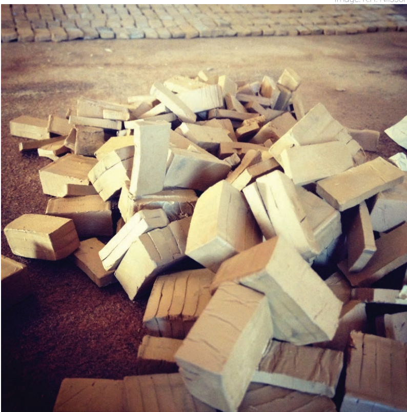
Brick tile production for model building, scaled 1:10, during the drying process before being burned in a kiln at 900 degrees Celsius.
