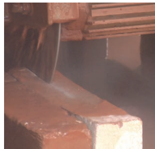
A lot of pre work had to be done. The tiles were salvaged from a refurbishment in an old house in Gothenburg and some from a demolished 19th century service building (Swedish: brygghus) and brought in by truck. All bricks were then cut into tiles.
