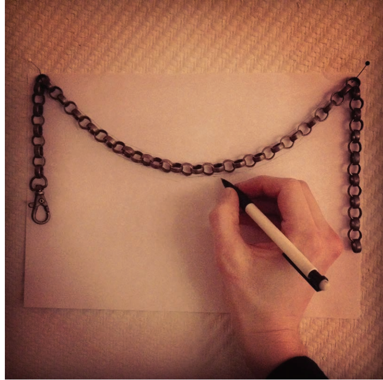
Above: A chain pinned to a wall is traced to find a funicular form.
