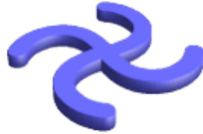
Figure 5: Example of design of a light-driven motor in a gammadion shape. The symmetry of the structure allows it to induce angular momentum from a linearly-polarized plane wave thanks to patterning of the phase retardation within the structure.
