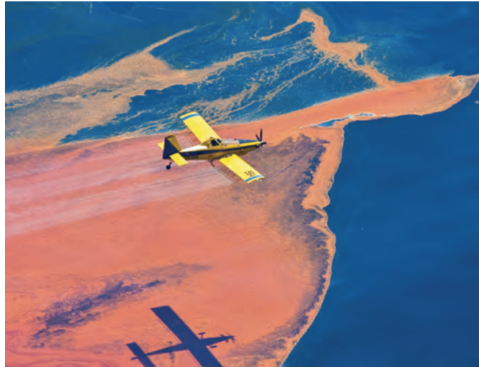
Figure 5.8 The use of Dispersants unloaded from an aircraft (ITOPF, 2013g, p.6).
