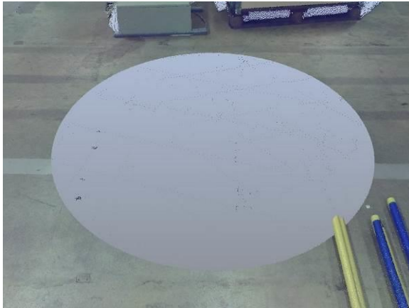
Fig. 6. The gap of scan data below the scanner.
