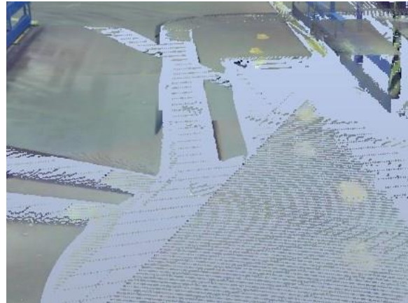
Fig. 7. Problem with insufficient amount of scan data.
