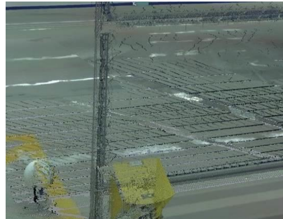
Fig. 11. Quality problems with scanning a lattice.
