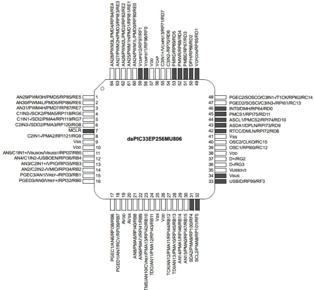
Figure 2.1: Pin diagram of dsPIC33E [8].
