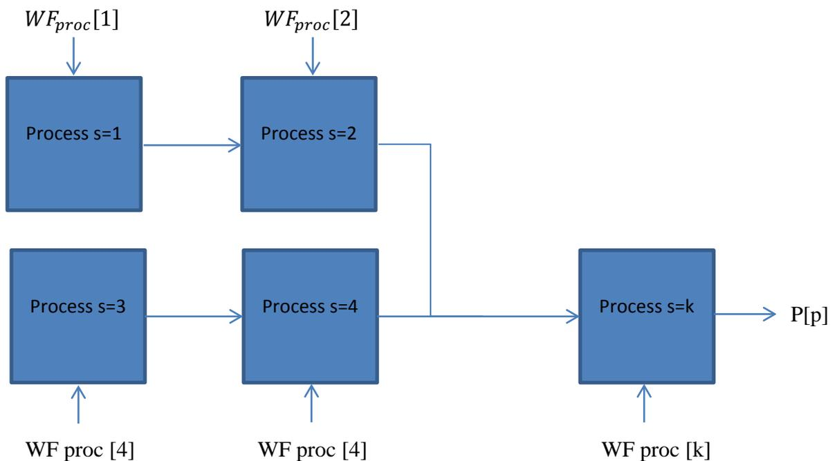
**Figure 2.** “Schematization of the production system to produce product  $p$  into  $k$  process steps, some steps are in series, others are parallel. The water footprint of output product  $p$  is calculated as the sum of the process water footprints of the processes that constitute the production system.” Source : (Hoekstra et al., 2011)
