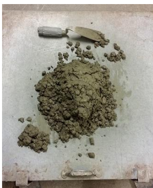
Figure 9: Concrete with no plasticiser.
