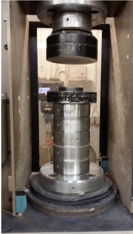
Figure 4: Image of the MTS machine showing the parts that measured compression strength.
