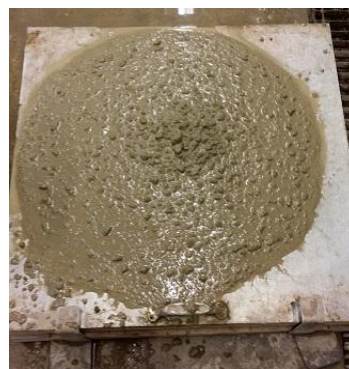
Figure 10: Concrete with too much plasticiser.
