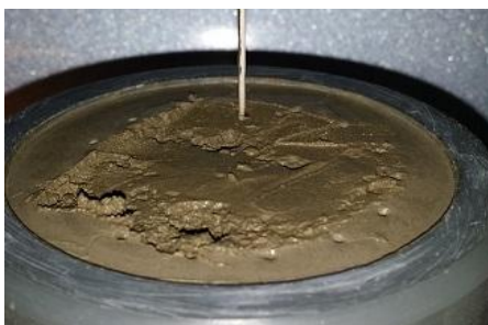
Figure 14: Top layer of 50 % cyclone ash mixture have been removed and shows holes in the paste.
