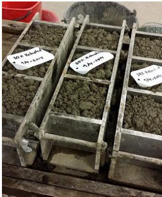
Figure 8: Mould for casting concrete cubes to be used in compression testing. In this case 9 cubes filled with unwashed 30 % wood ash mixture.
