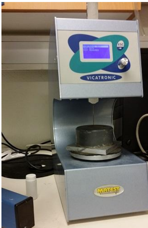
Figure 1: The Vicatronic machine used to measure setting time and picture was taken during a test.
