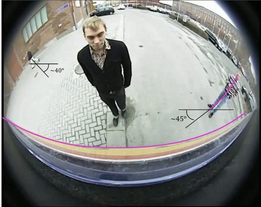
**Figure 1.5:** A captured frame from the camera system that displays the vertical rotation (highlighted in black) and the significant non-rectilinearity of objects (highlighted in fuchsia) caused by radial distortion.
