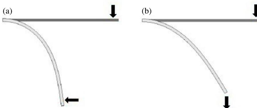
**Figure 5.1** The principal difference between loads of a non-linear analysis (a) and a linear analysis (b). Dassault Systèmes, (2008)
