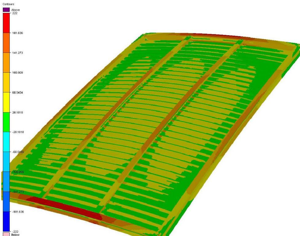
**Figure 2** *Von Mises stresses in the car deck structure, bottom view.*
