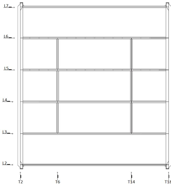
**Figure 2.4** The supporting frame and grid system of the centre reference deck.
