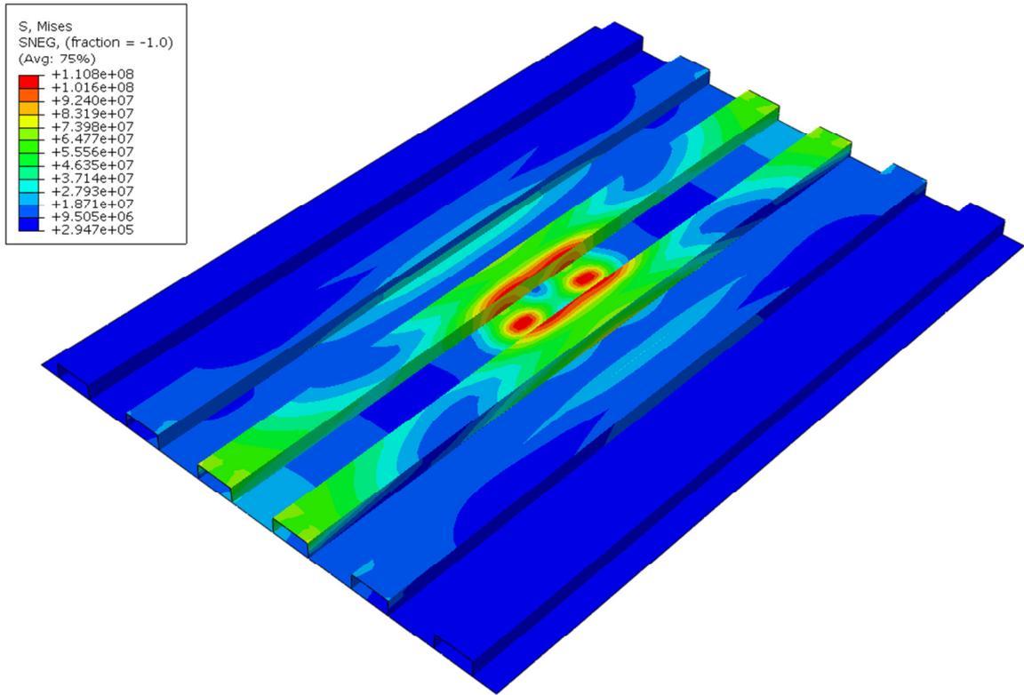
**Figure 9** Von Mises stresses, LC2.
