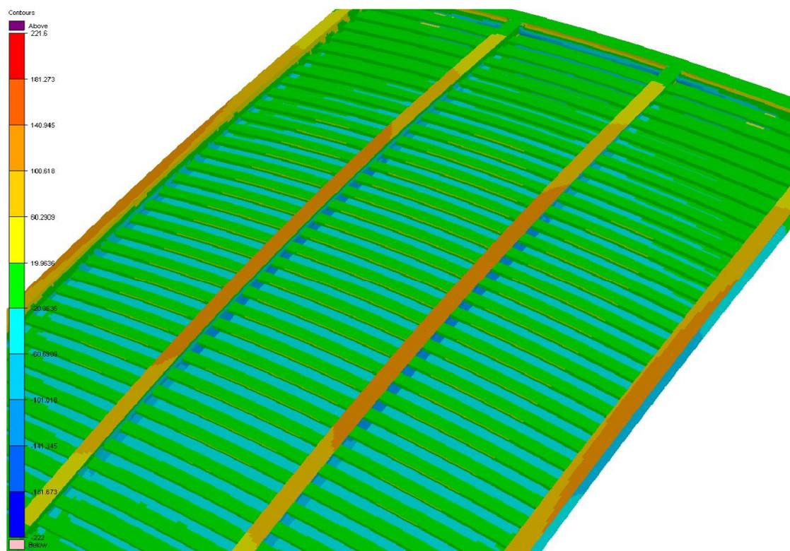
**Figure 4** Normal stresses in the longitudinal stiffeners.
