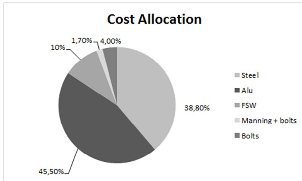
**Figure 7.2** Cost allocation of the side car deck panel
