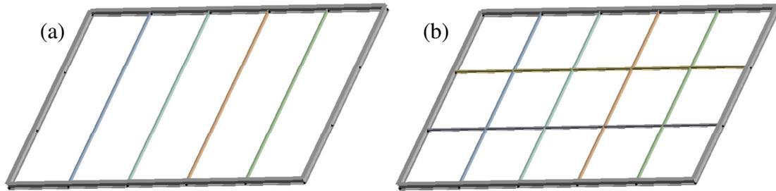
**Figure 4.4** *Transverse stiffener: Concept (a) has no transversal beams, making it ideal for keeping manufacturing costs low. This concept also has the potential of reaching the lowest mass. Concept (b) has two transversal beams, which allows the structure to reach a lower deflection, with the cost of higher mass.*
