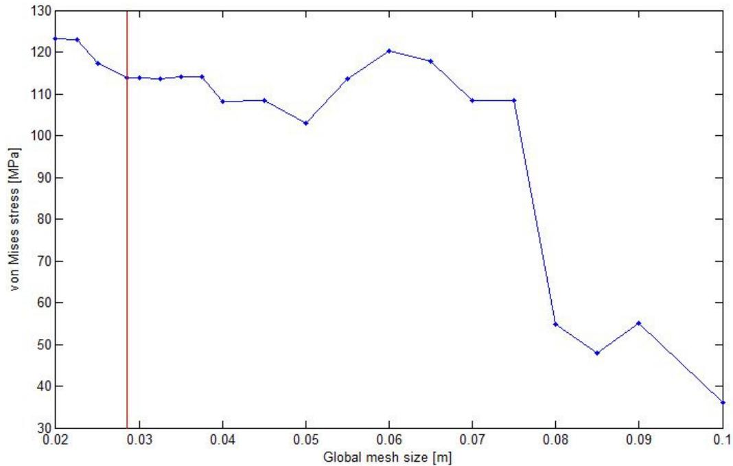
**Figure 5.3** Convergence study for the Abaqus model.
