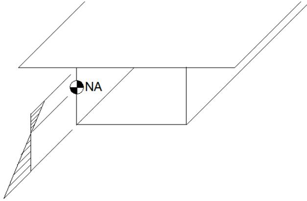
**Figure 3.2** The normal stress distribution due to bending.
