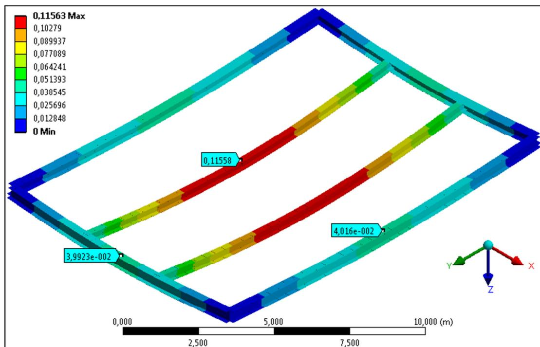
**Figure 6.9** Vertical deflection of the side car deck panel.
