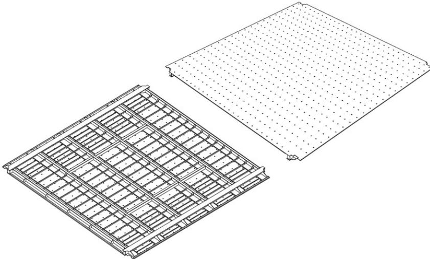
**Figure 2.3** Conventional car deck solution.
