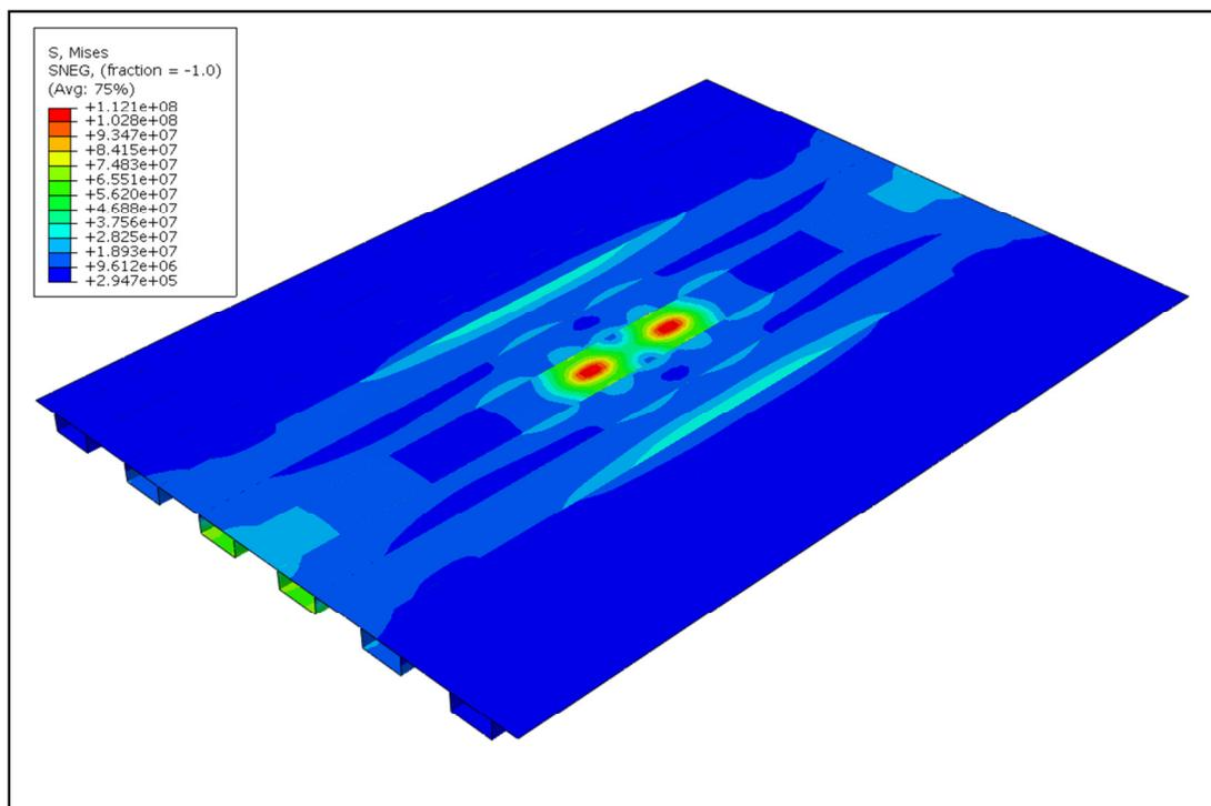
**Figure 6.3** The Von Mises stresses in the stiffened top plate due to the tyre load.
