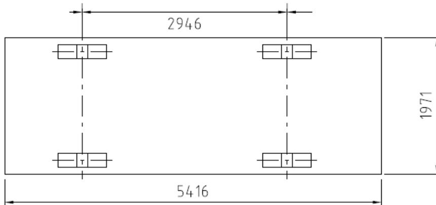
**Figure 5.5** Dimensions of the car used for determining the distance between tyre prints in load case 3.
