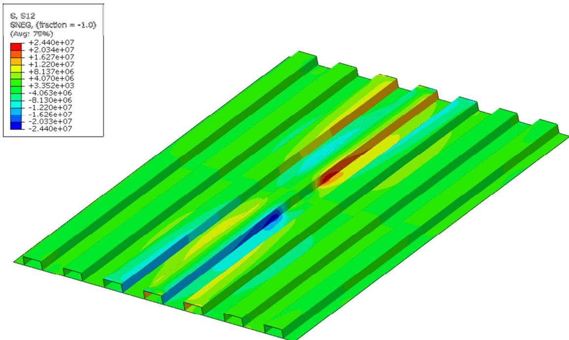
**Figure 6** Shear stress, LCI.
