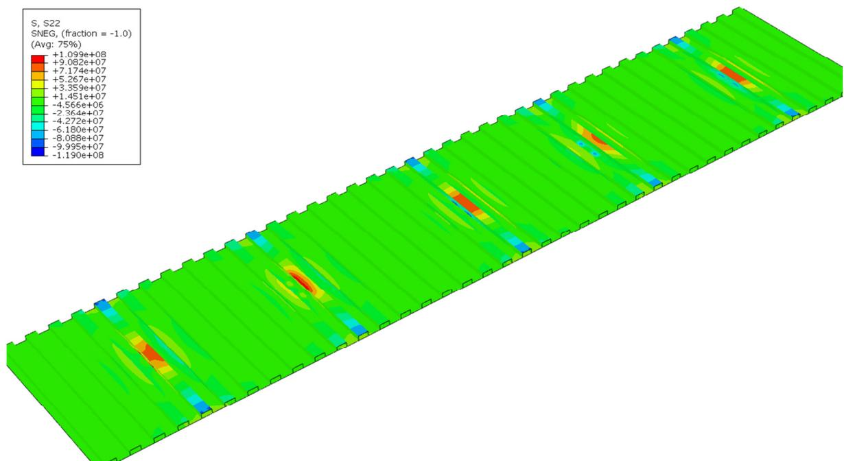
**Figure 18** Normal stress in the stiffeners for load case 3. The negative stress of 119 MPa occurs in the web, in this model this is not the normal stress since the S22 direction of that structural member is not normal to the cross-section, this can be seen in Figure 19. Hence, this is disregarded.
