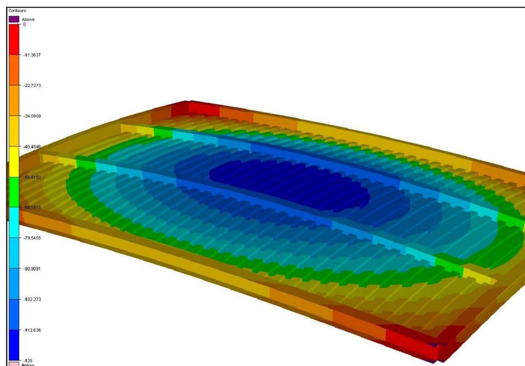
**Figure 6.10** The deflection of the car deck panel.
