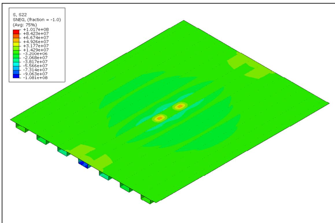
**Figure 6.7** The normal stress in the stiffened top plate for load case 2.
