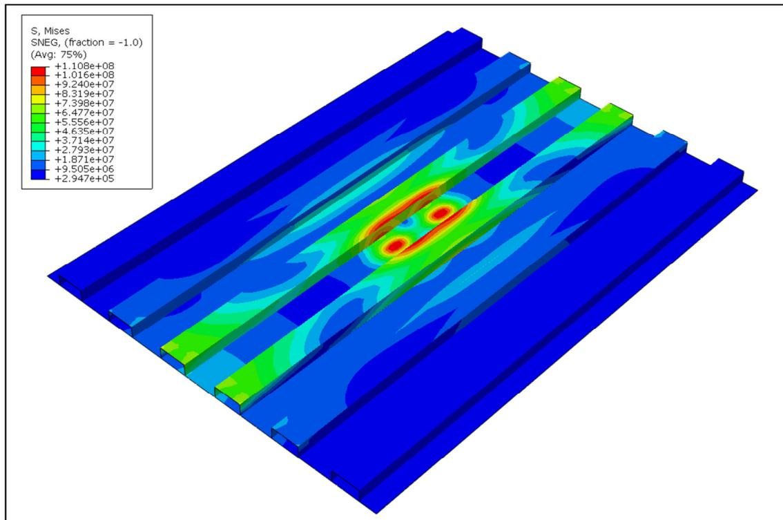
**Figure 6.4** The Von Mises stresses in the stiffeners due to the tyre load.
