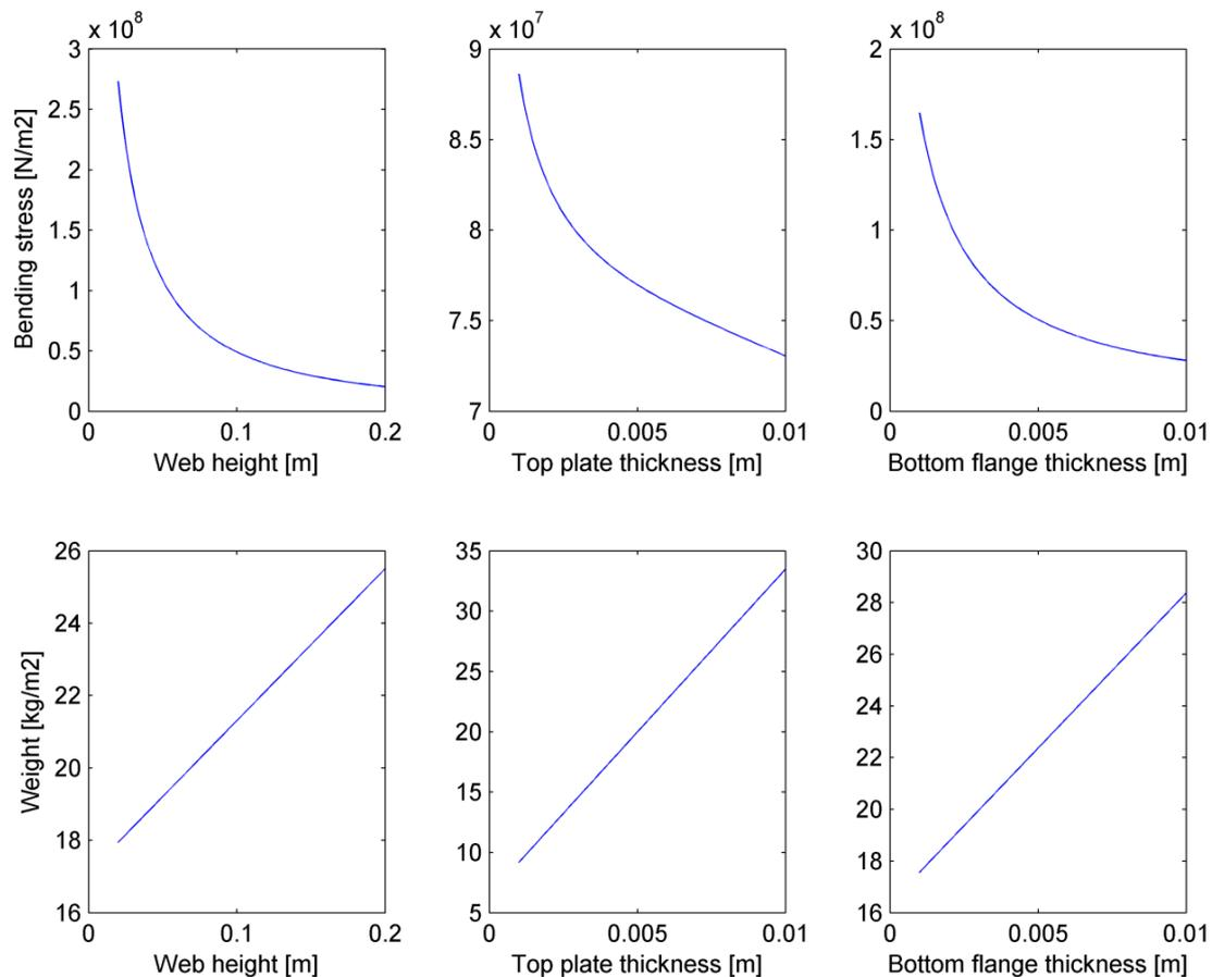
**Figure 4.3** Bending and weight depending on web height, upper and lower plate thickness. In the graphs, all dimensions are set according to the end design, except for the variable under study.
