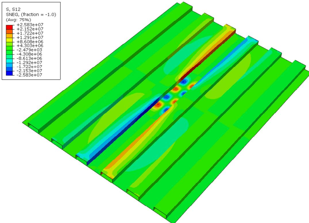
**Figure 12** Shear stress, LC2.
