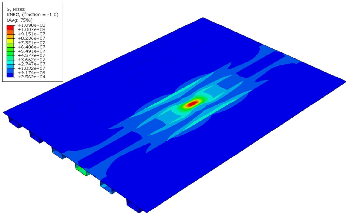
**Figure 7** Von Mises stress, in the top plate between webs, from one tyre turned 90 degrees, LC1.
