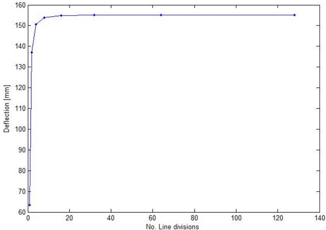
**Figure 5.6** The result from the convergence study, showing deflection (mm) for different number of line divisions
