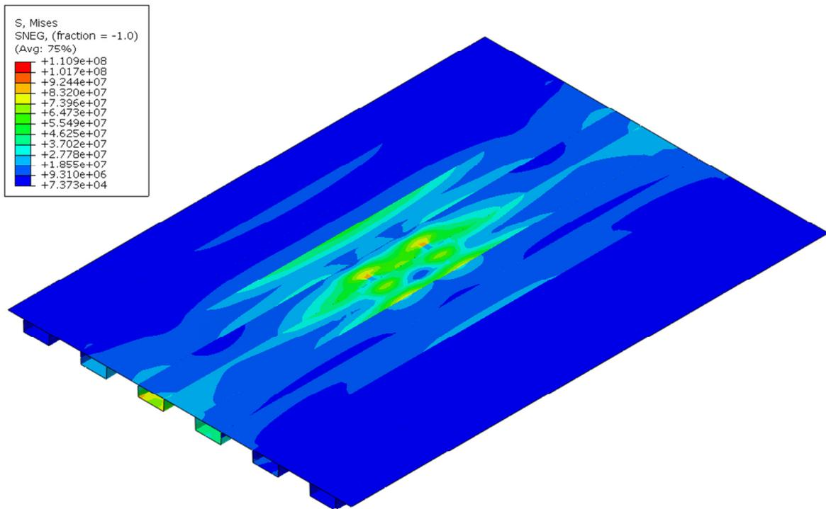
**Figure 14** Von Mises stresses due to the load from two tyres placed on the weld.
