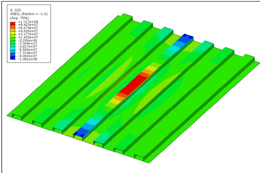
**Figure 6.6** The highest normal stress that occur in the panel.
