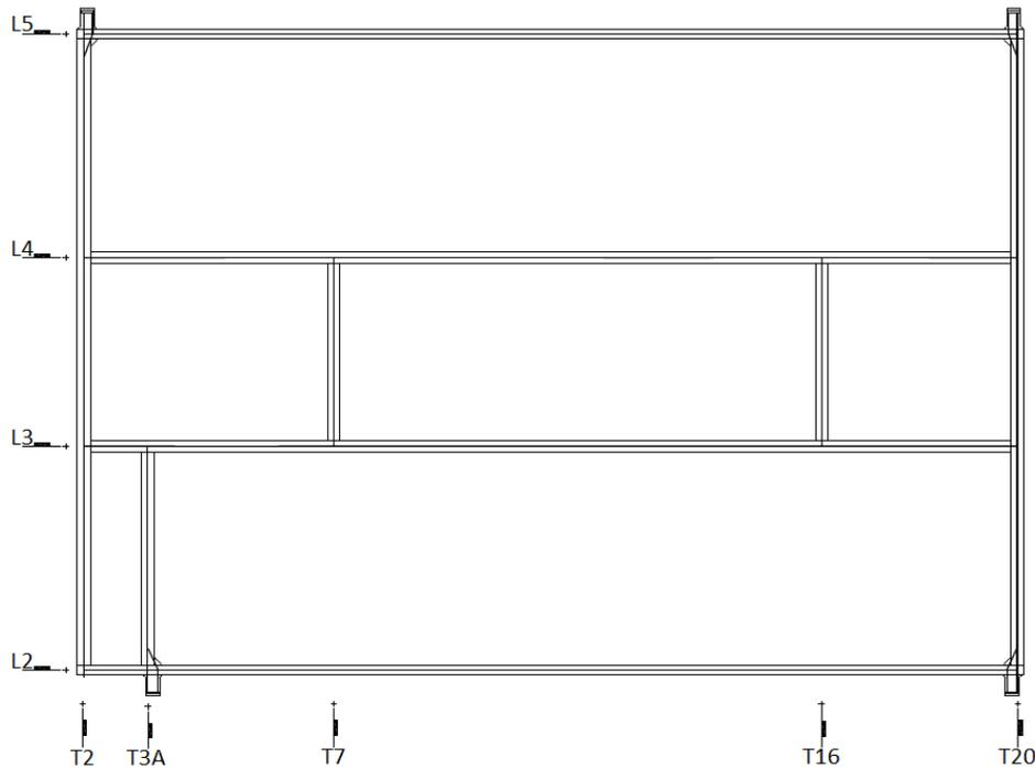
**Figure 2.5** The arrangement of the supporting structure for the side car deck reference solution.
