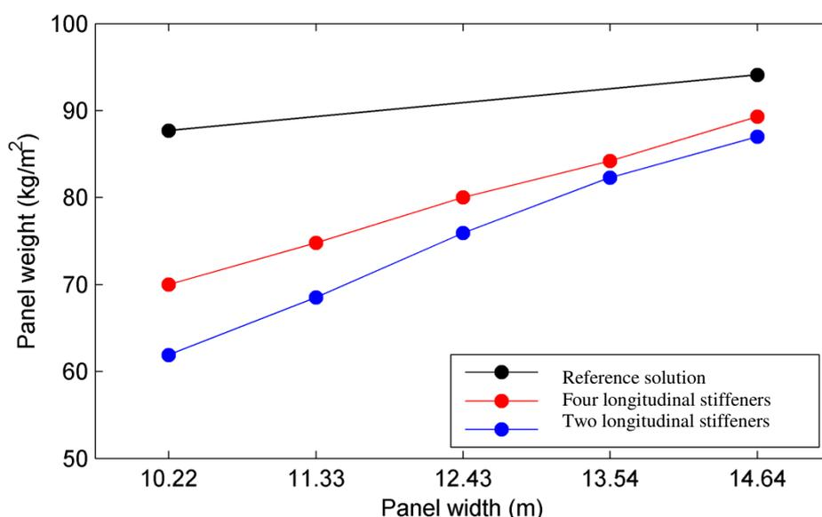
**Figure 7.1** Weight per area for different sizes of car decks.
