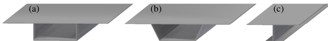
**Figure 4.2** Concepts of extruded aluminium: a) Concept #1: Vertical webs with closed cross-section, making this concept good from a weight-perspective and resilient to buckling. b) Concept #2: Webs inclined with an angle and closed cross-section, making this concepts ideal for resist buckling but of the cost of slightly higher mass. c) Concept #3: Vertical, single-web cross-section, making this concept ideal for reaching low weight solutions, but of the cost if higher risk for buckling.
