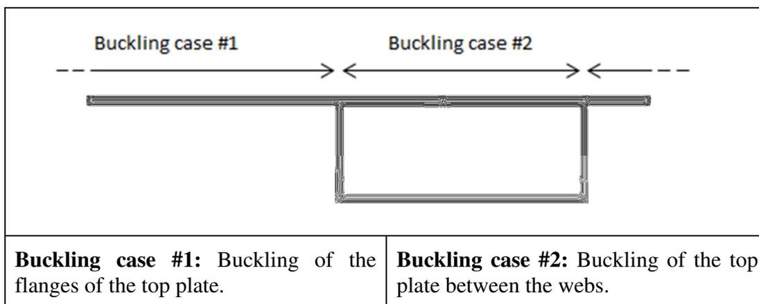
For both buckling cases, the concerned area is considered a plate. The profiles are bolted in the ends and can therefore be considered as fixed supports. As long as bolts don't get loose, the profile is fixed. Hence, according to Ringsberg, (2011) the critical buckling stress can be calculated as in Equation 3.5
