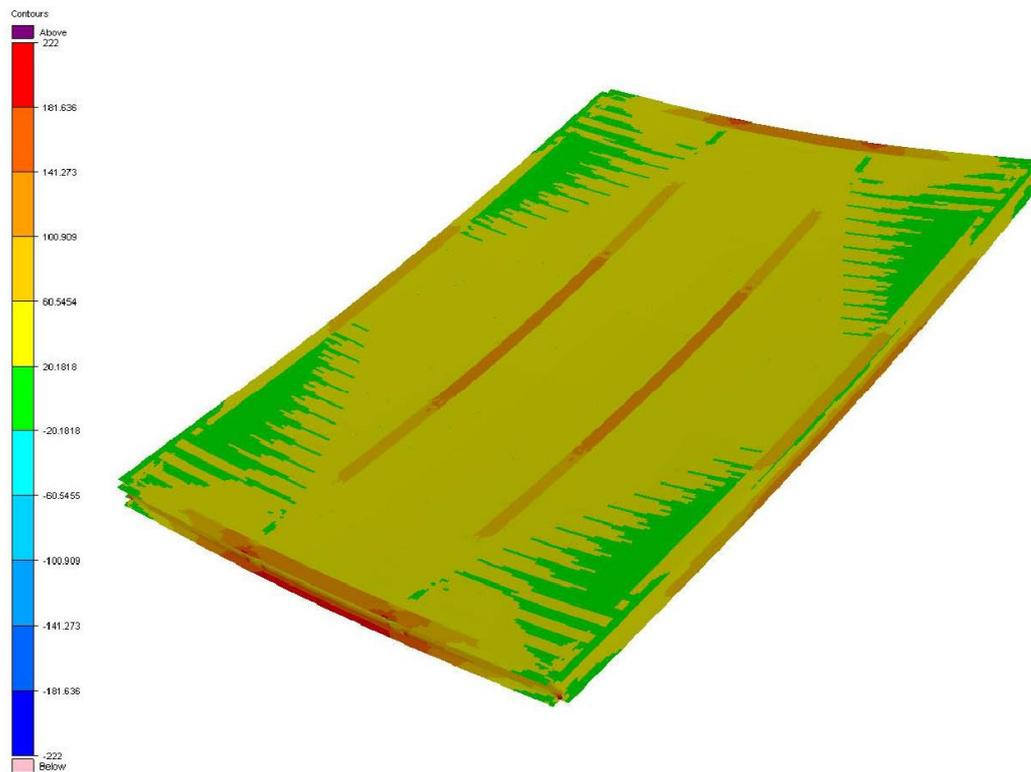
**Figure 1** *Von Mises stresses in the car deck structure, top view.*
