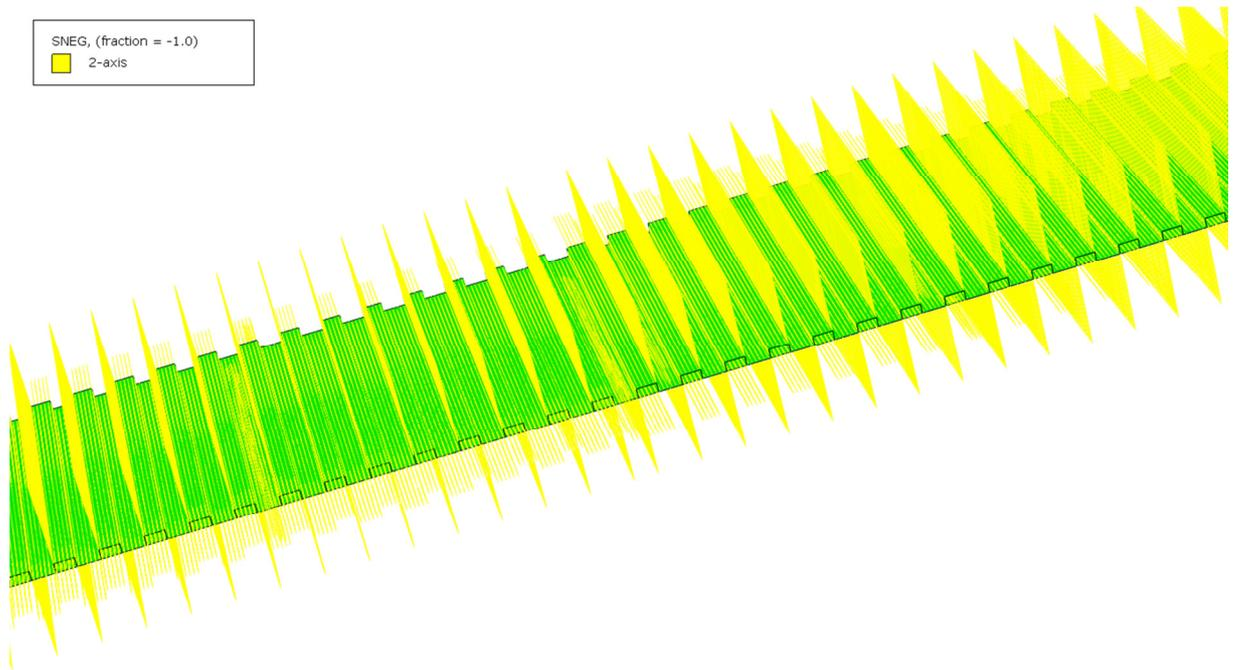
**Figure 19** *S22 direction for the structural members, here the S22 of the flange and top plate is normal to the cross-section while the S22 of the webs are not.*
