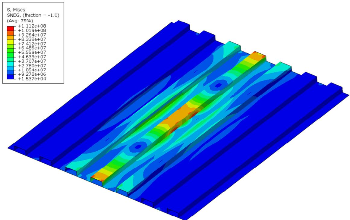
**Figure 2** Von Mises stress, LCI
