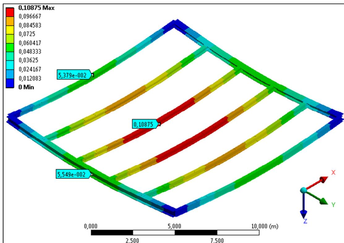
Figure 6.8 Vertical deflection of the centre car deck panel.
