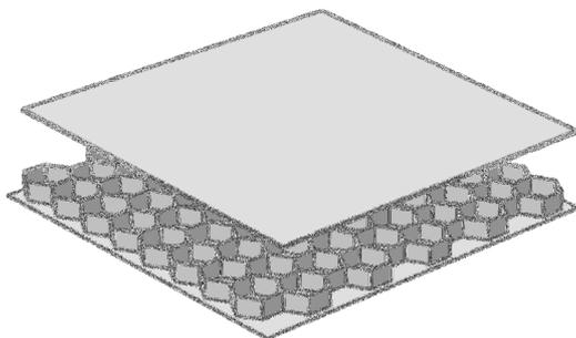
**Figure 4.1** *Honeycomb sandwich structure*
