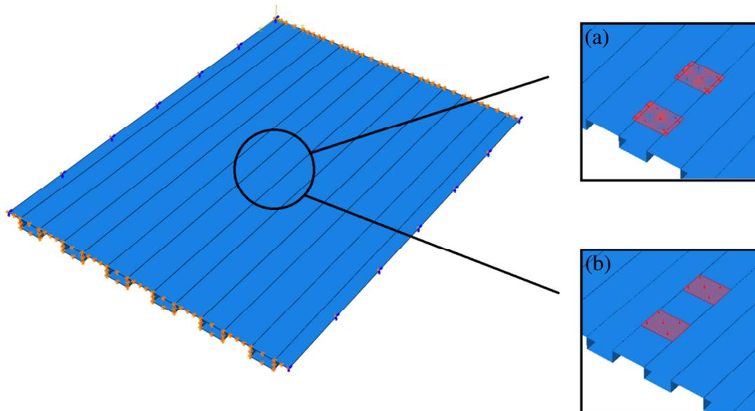
**Figure 5.2** The two different load cases studied in the FE-analysis.
