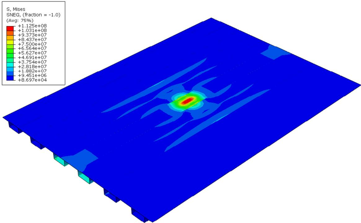
**Figure 13** Von Mises stress, in the top plate between stiffeners, from one tyre turned 90 degrees, LC2.
