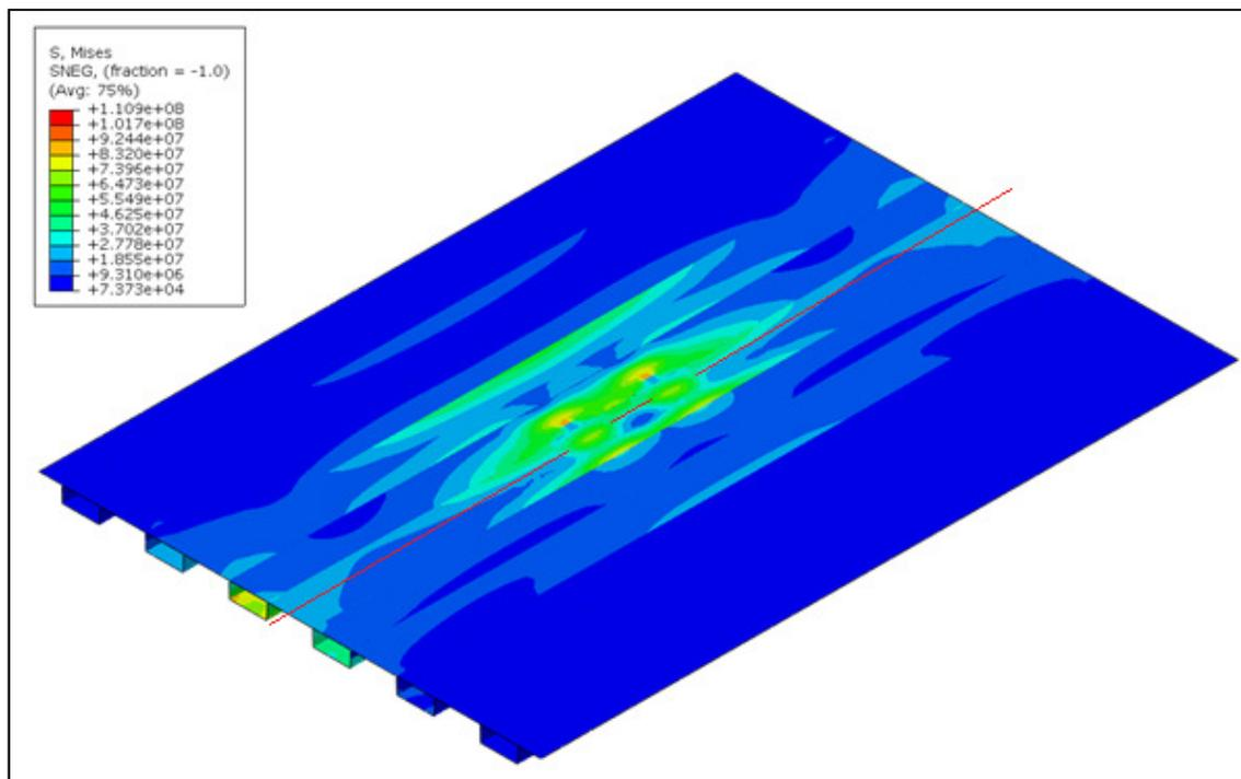
**Figure 6.5** The highest stresses that will occur at the weld due to the tyre load.
