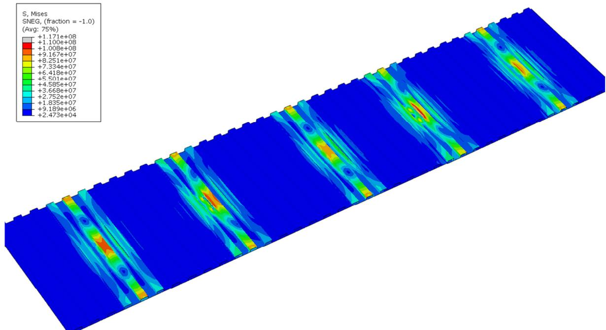
**Figure 17** Von Mises stress in the stiffeners for load case 3.
