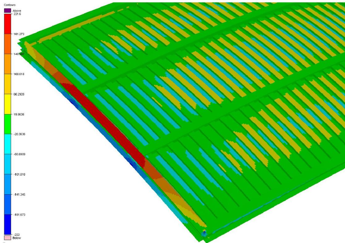
**Figure 3** Normal stresses in the load bearing frame.
