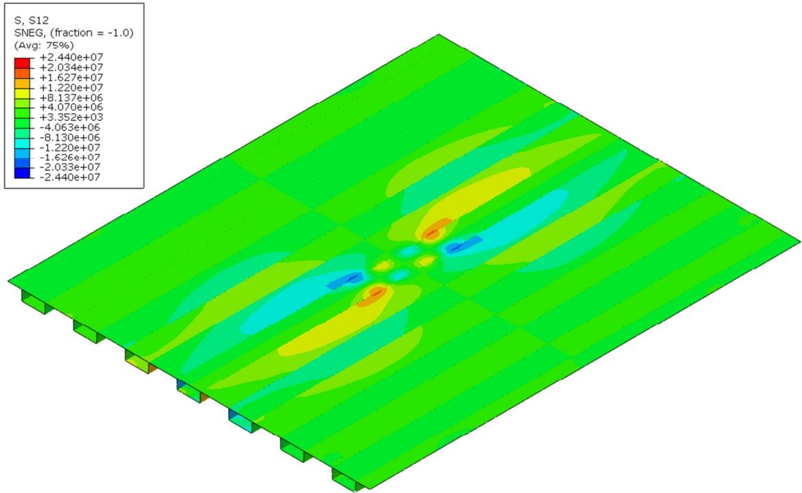
**Figure 5** Shear stress, LCI.
