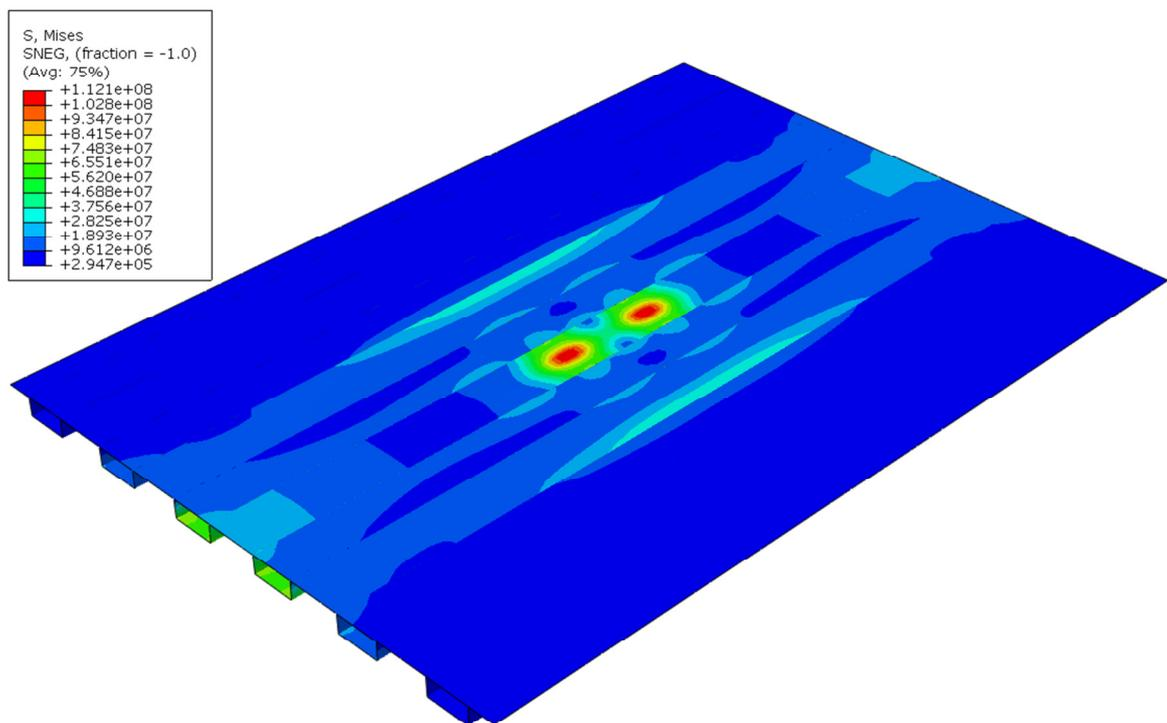
**Figure 8** Von Mises stresses, LC2.
