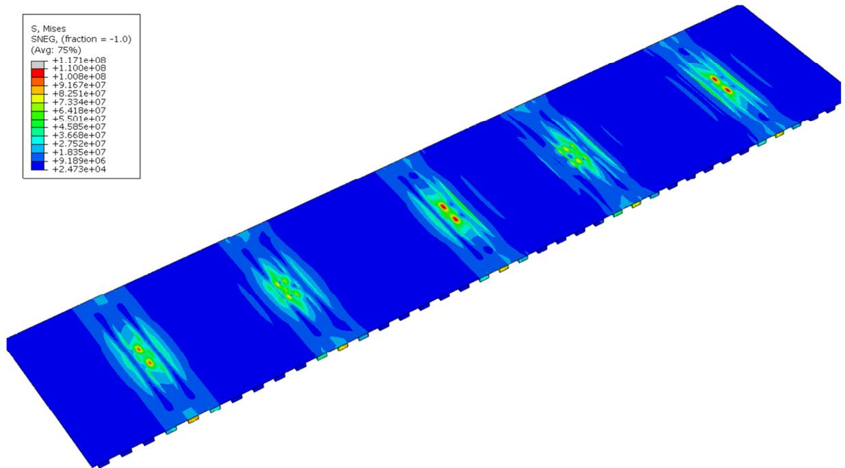
**Figure 16** Von mises stress in the stiffened top plate for load case 3.
