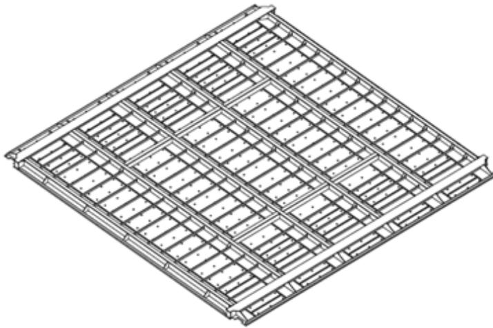
**Figure 1.1** *Structural arrangement of a conventional car deck.*
