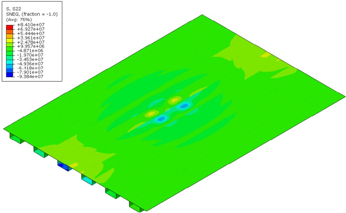
**Figure 15** Normal stresses due to the load from two tyres placed on the weld.
