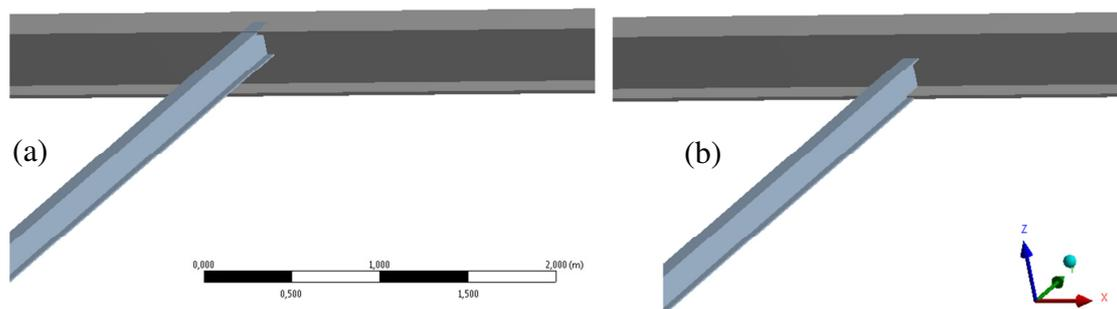
**Figure 4.5** *Longitudinal stiffeners attached on upper flange (a) and on lower flange (b) of the frame.*
