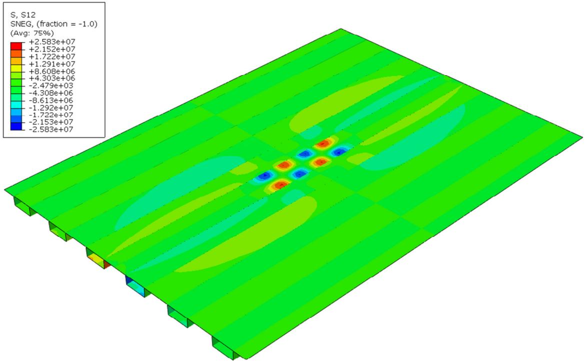
**Figure 11** Shear stress, LC2.
