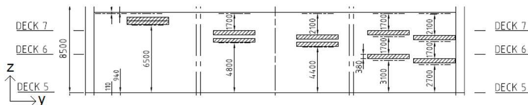
**Figure 2.2** Different configurations of the liftable car deck panels.
