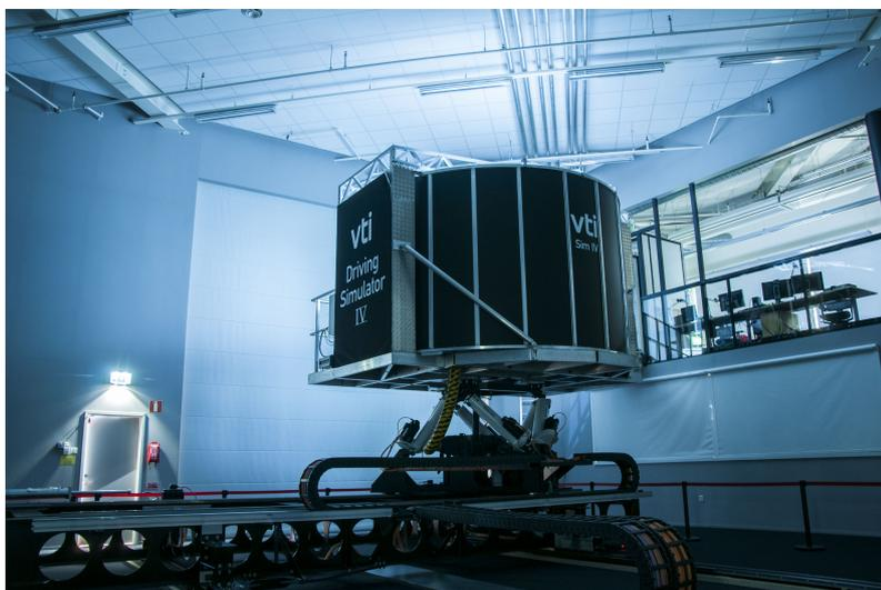
Figure 4.1: The VTI Sim IV driving simulator, dome and motion system.
