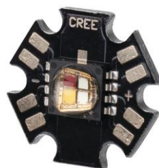
Fig 6.4. Power LED with integrated red, green, blue and white diodes
