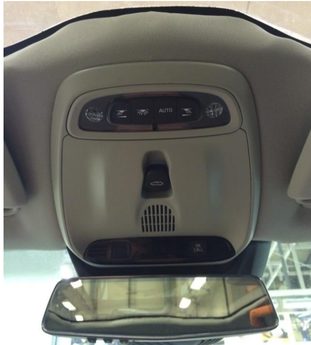
Fig 4.2. The current overhead console, containing both general and located lighting
