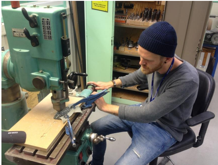
Fig 6.12. Milling tracks through the plastic of the Clean Air Indicator
