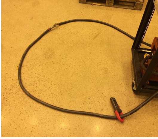
Figure 3.21 Circular orientation for maximum inductance.
