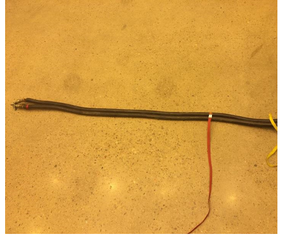
Figure 3.22 Tight orientation for minimum inductance.
