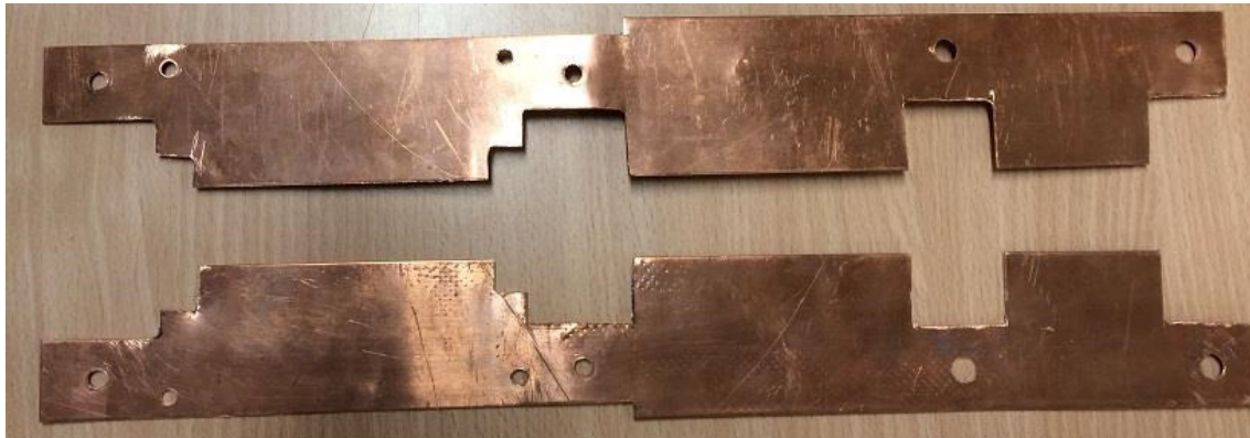
Figure 4.7 Copper plates of the dc-link.
