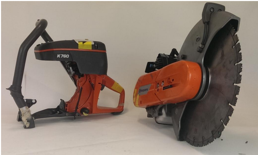
Figure 1.4. The power cutter divided into its main parts.
