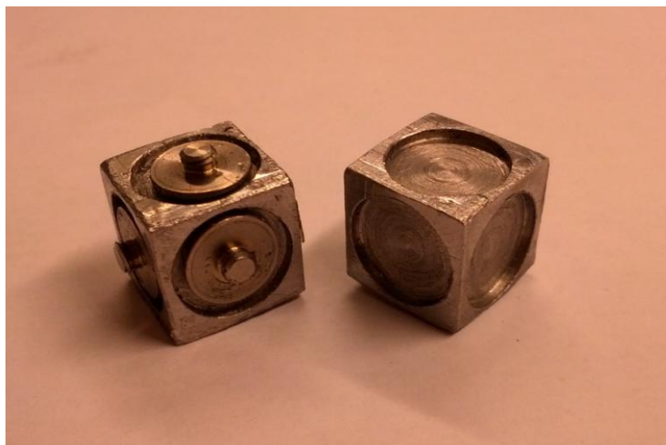
Figure 4.6. The mounting brackets used to achieve perpendicular accelerometer placement.
