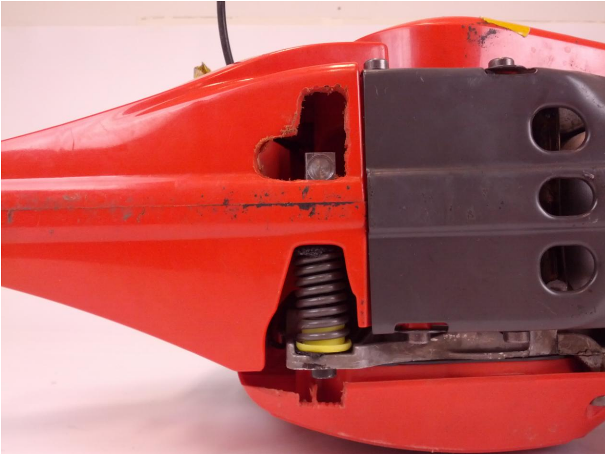
Figure B2. The mounting bracket inside the tank. At the bottom of the picture plastic has been removed to accommodate for the mounting bracket on the air intake.
