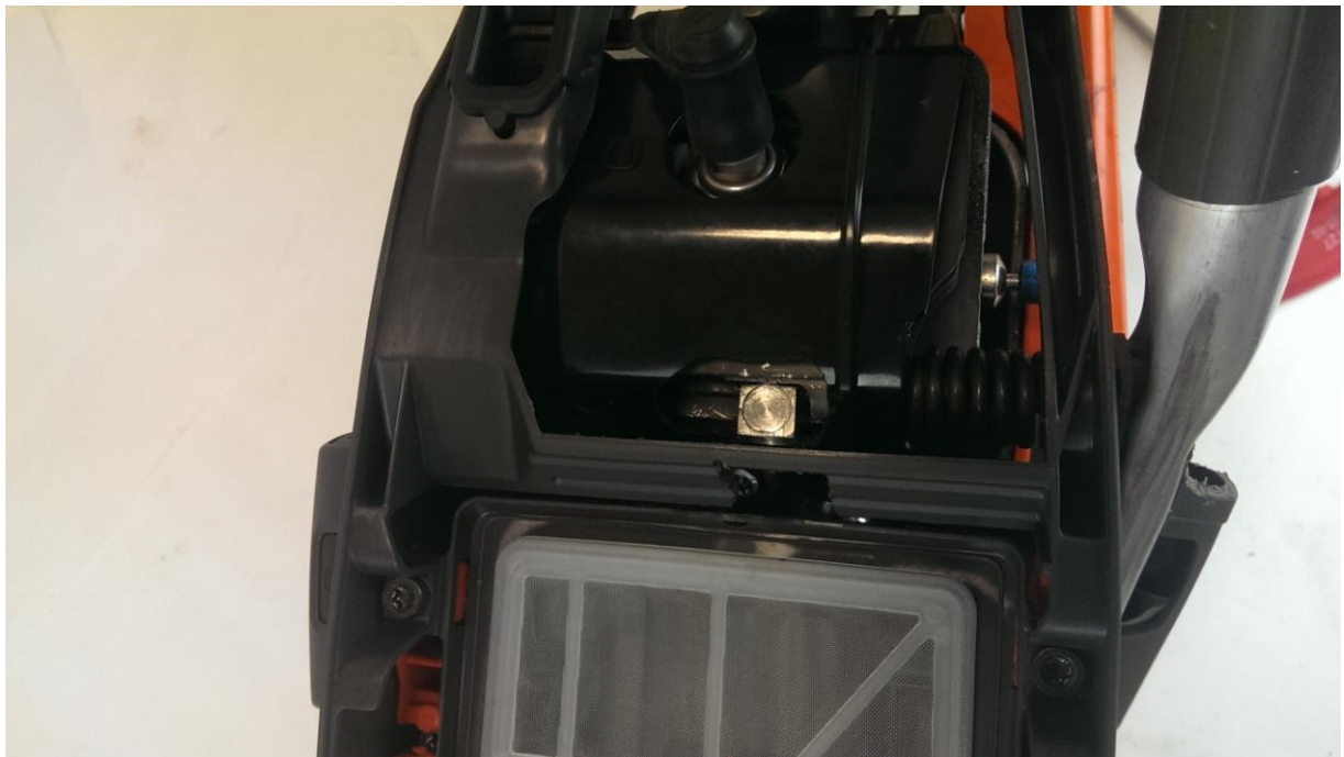
Figure B3. The mounting bracket on the engine.
