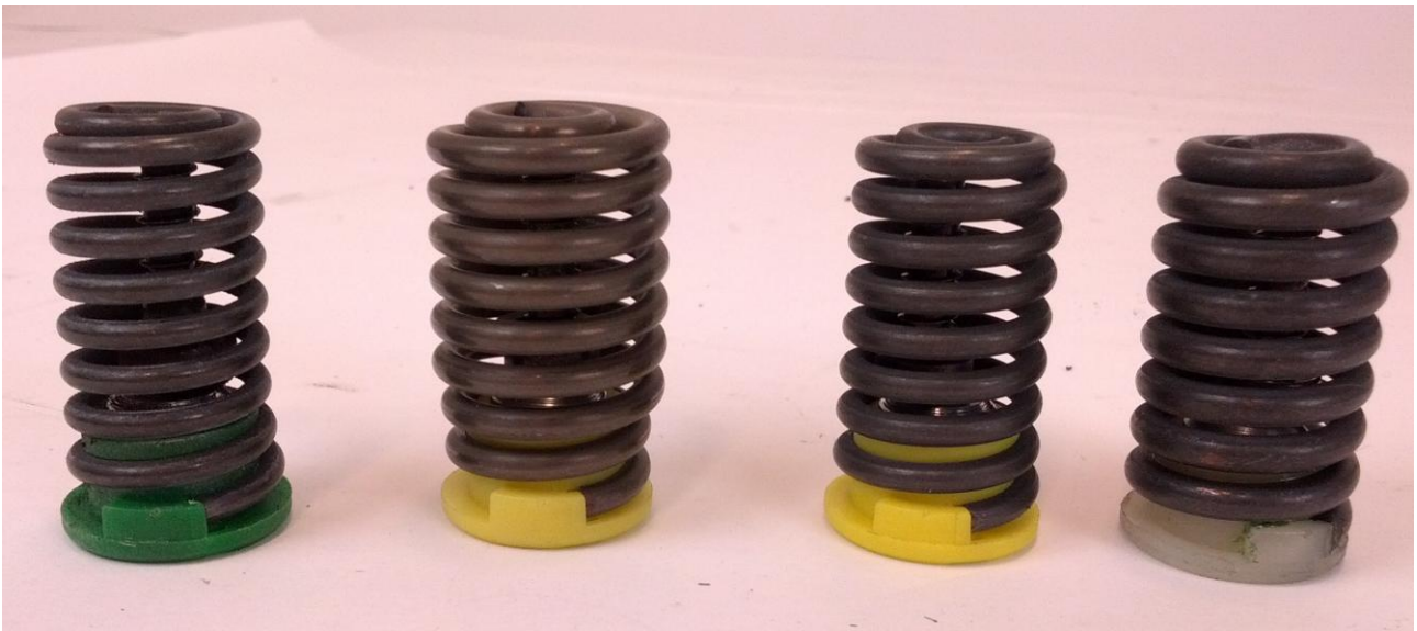
Figure 3.2. The different springs that were tested. From left to right: Weak, prototype, standard and stiff.
