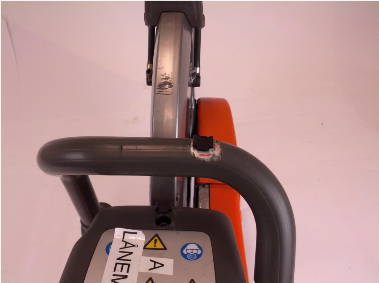
Figure B4. The mounting bracket for the three-axis accelerometer on the forward handle.
