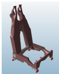
Inspire: suggests material at outer ends, upper section needs less material
