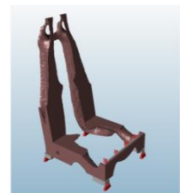
Inspire: Still needs material at outer ends, nothing needed in the center due to the increased stiffness of a one-piece design (Inspire suggests 60 % reduction in mass)
