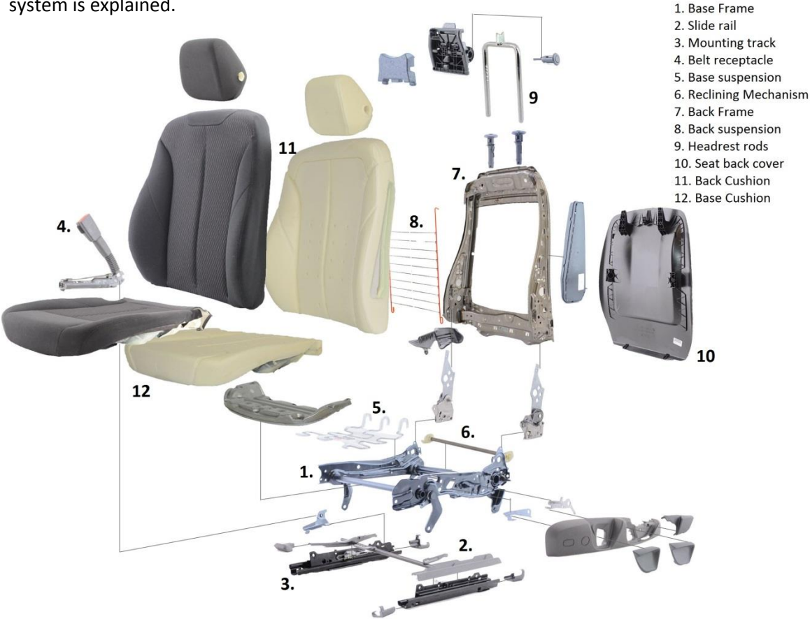
Figure 2: Exploded view of a typical modern car seat, BMW 3 Series 328i (A2mac1 2014)
