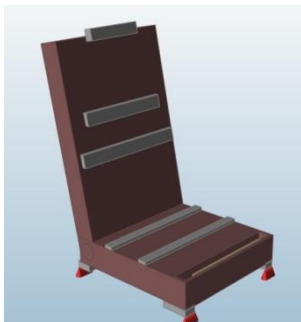
Figure 28: Initial design domain for the fixed seat structure concept.
