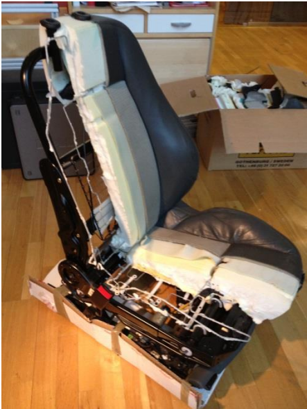
Figure 7: The reference seat halfway through the reverse engineering process
