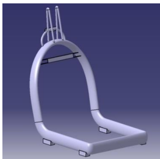
Figure 30: Topology optimized design modeled in CATIA.
