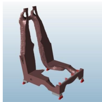
Figure 29: Topology optimized design of the fixed seat structure concept. Suggesting 60 percent mass reduction compared to reference design.
