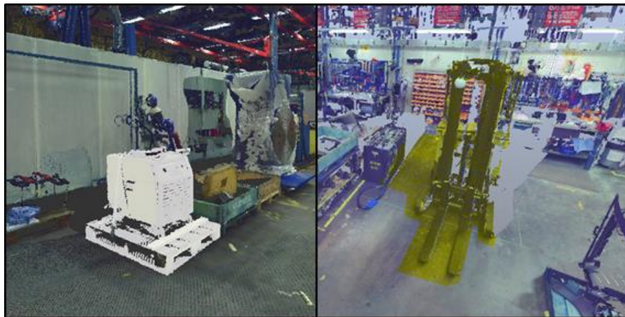
Figure 8: Examples of point selection in ReCap (left) and Scene (right), selected points are white and yellow respectively.
