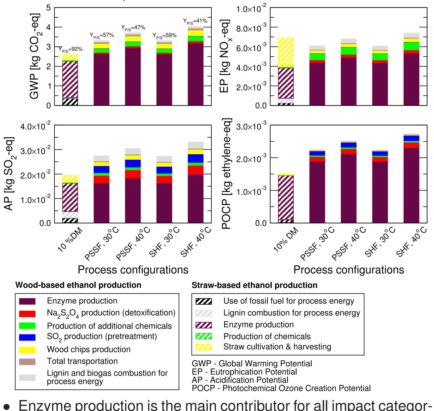
velopment for the production of ethanol from wood and straw<sup>2,3</sup> using experimental data
