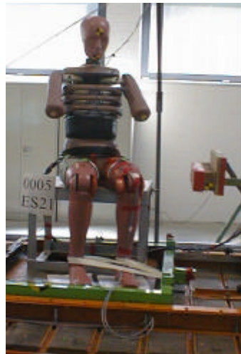
Figure 16: ES-2 prototype and EUROSID-1 in sled tests at BAST. Impact speed 20 km/h; Impact direction 20 degrees forward (knee contact first) , Left: Test set-up. The barrier is a padded bar covering pelvis, upper leg and knee. Right: ES-2 prototype and EUROSID-1
