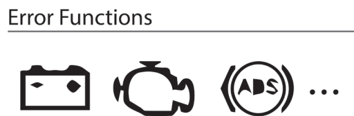
Fig 19: The error functions concerns battery not functioning as well as engine and brake problems.
