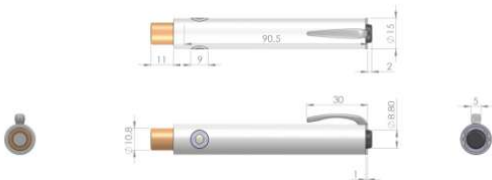
Figure 12.4. Dimensions of Electra Fusion with cap off, orange needle cover visible
