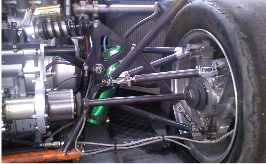
Figure 4.10: Example of push rod on double wishbone arrangement as on Chalmers Formula Student car 2012 (rear, driven).
