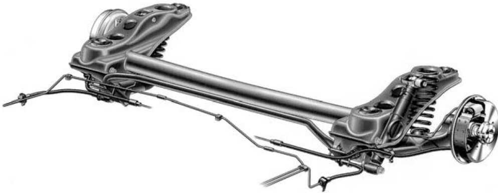
Figure 4.8: Example of a trailing arm suspension as on the Mercedes-Benz A class Mk1 (rear, non-driven). The lateral round beam is a part of the rear subframe. [7]
