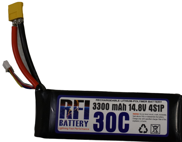
Figure 3.12: Battery 14.8 V 3300 mAh
