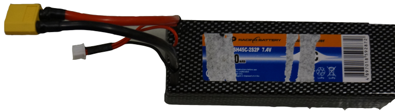
Figure 3.11: Battery 7.4 V 3300 mAh
