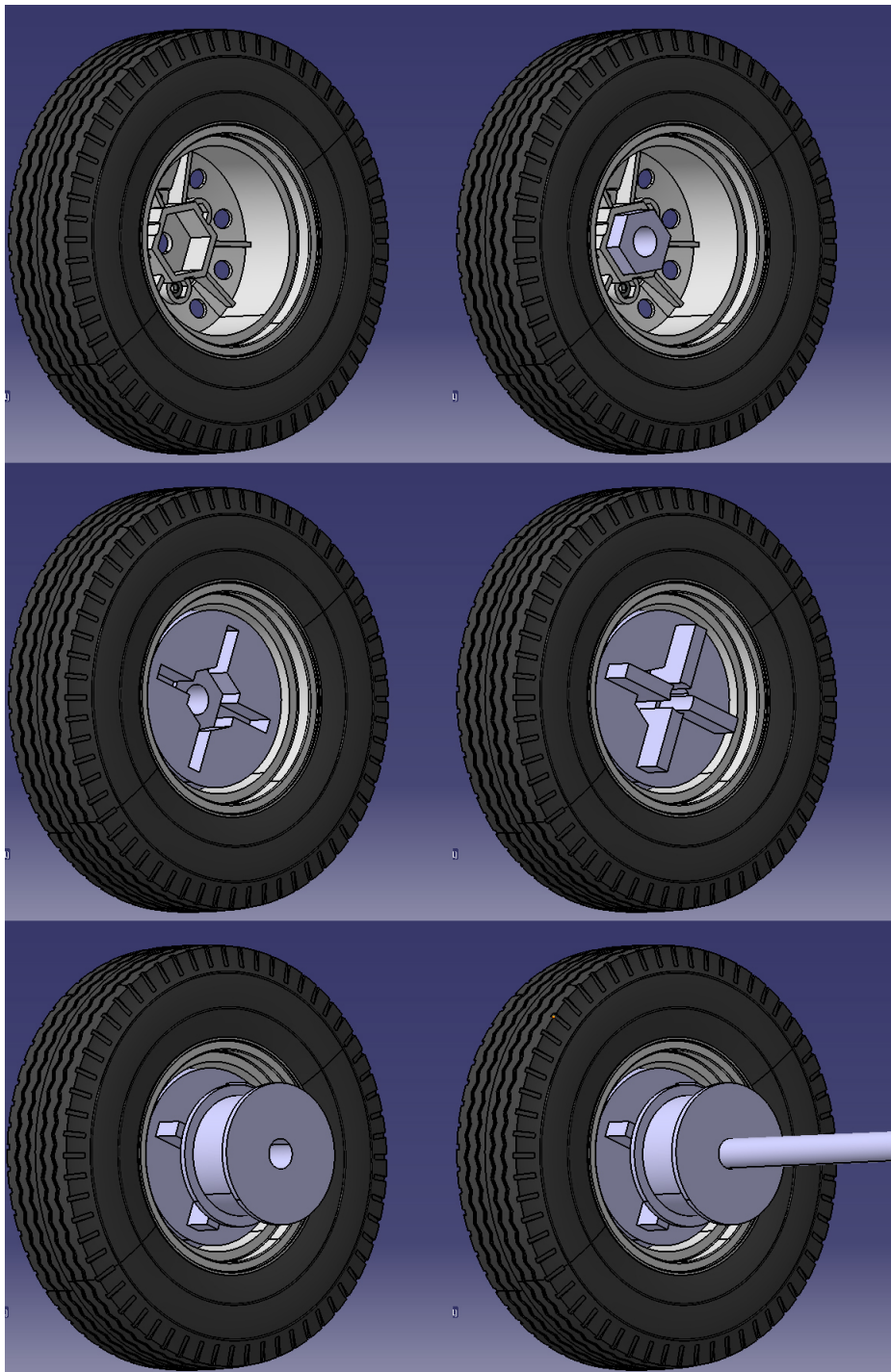
Figure 4.7: Assembling of the free adapter
